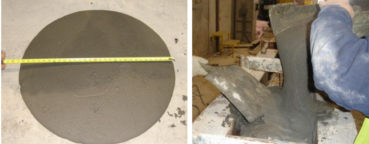
Figure 5.4 Flowability of NU UHPC Mix #4' Used for AASHTO Type II Girder B
