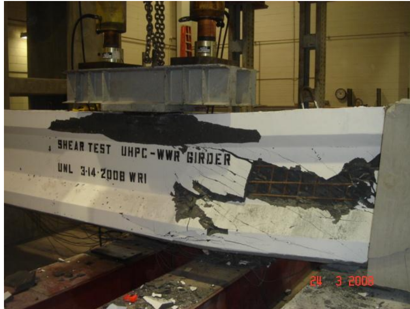
Figure 5.10 Failure of Girder B
