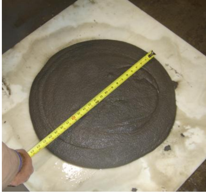
Figure 5.3 Flowability of NU UHPC Mix #4' Used for AASHTO Type II Girder A
