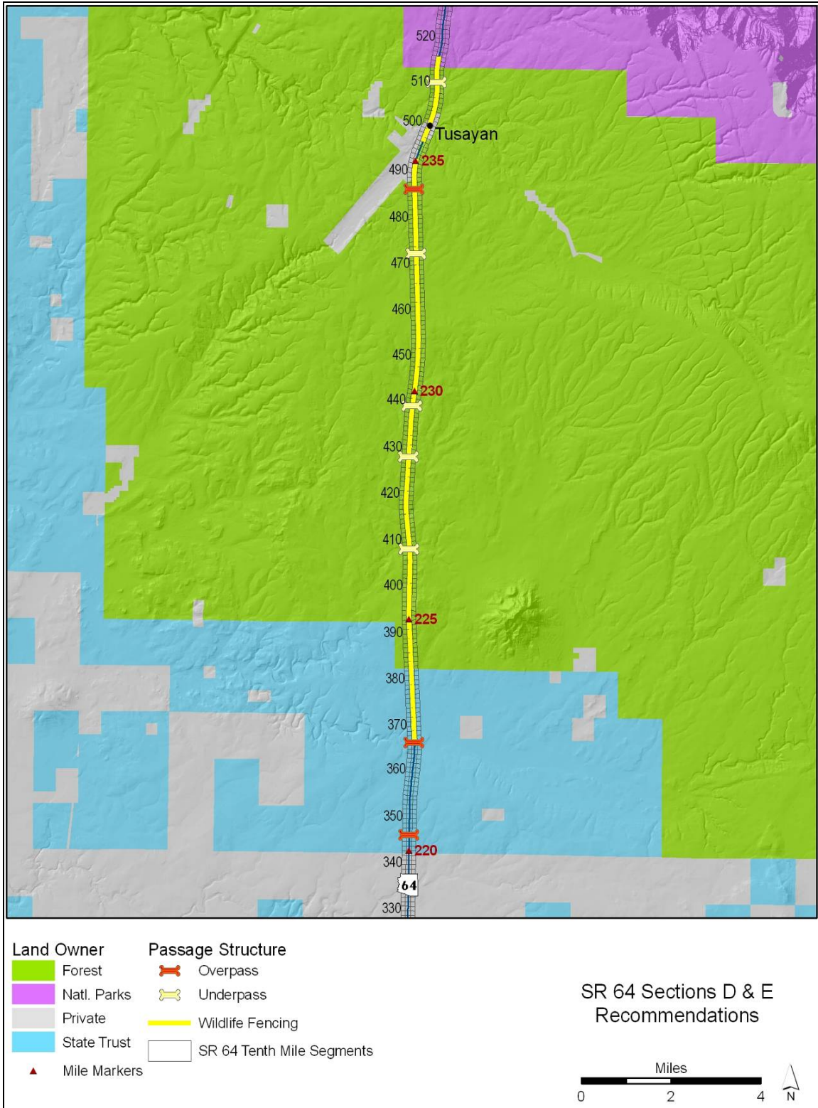
Figure 26. Recommendations for SR 64 Wildlife Passage Structures and Wildlife Fencing for Highway Sections D and E.
