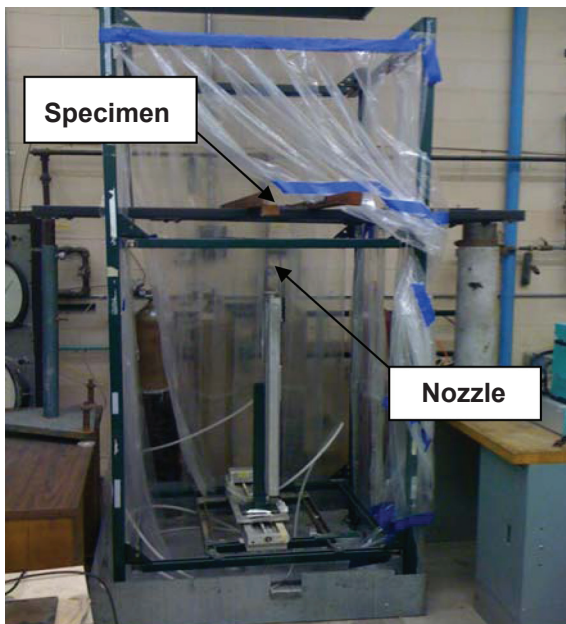
Jet flame test setup.
