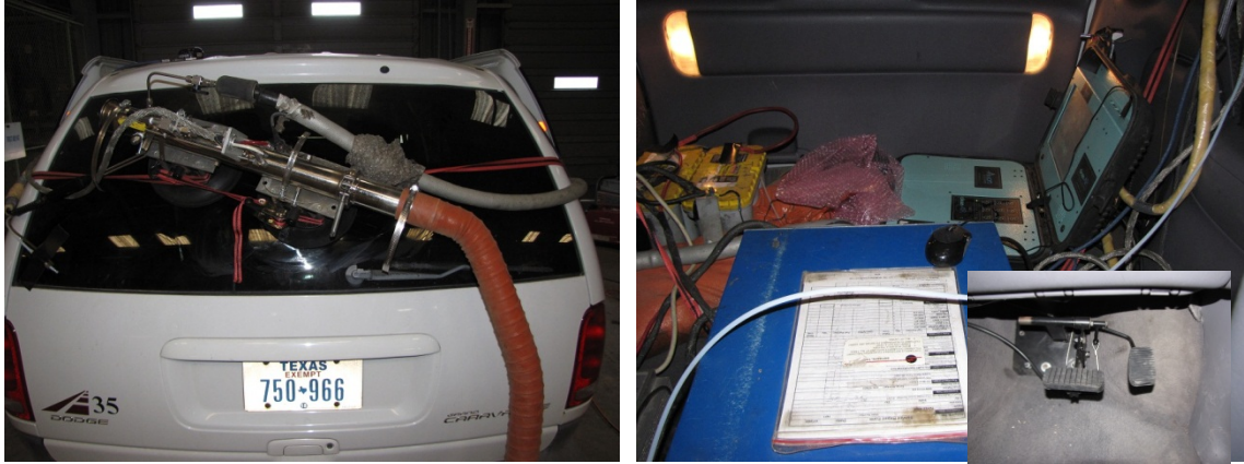
Figure 10. Test Vehicle Installed with PEMS (Left: Sampling Probes and Tubing Installed on Test Vehicle and Connected to Vehicle Exhaust, Right: SEMTECH-DS and Axion in Test Vehicle).
