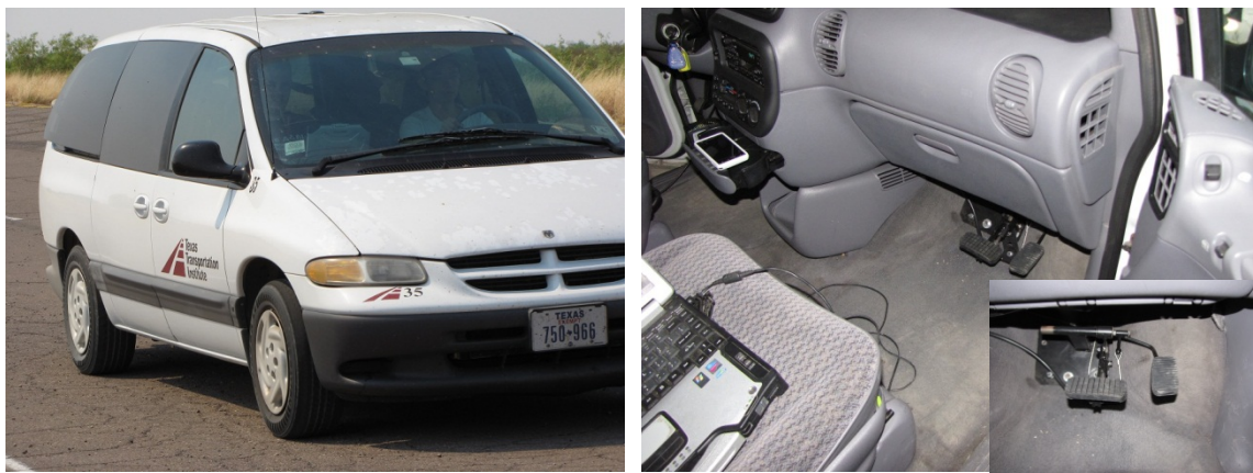
Figure 6. Test Vehicle (Left) and Slave Pedals in the Assistant Seat of the Test Vehicle (Right; Closed-up Pictures of the Pedals Are Also Shown in the Bottom Corner at Right).
