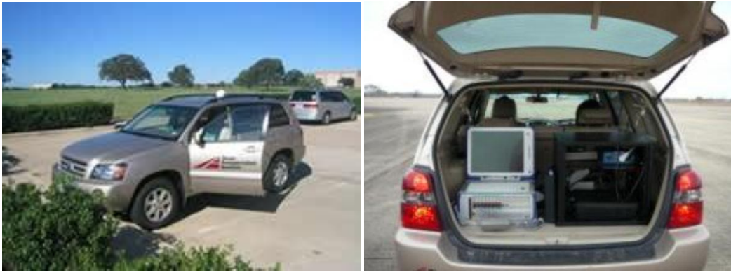
Figure 33. Instrumented vehicle and Dewetron DEWE5000 data acquisition system
