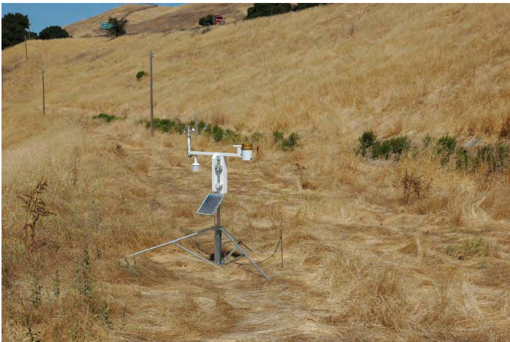
Figure 4. Evaporation measurement station at Contra Costa highway 4.
