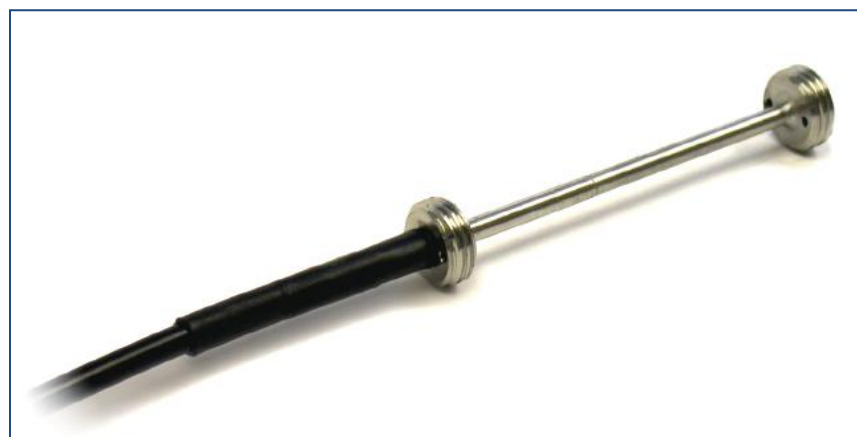
Figure 9: FISO EFO fiber optic strain gauge (FISO, 2008)
