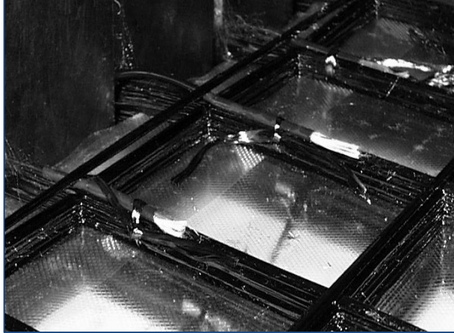
Figure 11: Strain sensors embedded in NEFMAC grid (Adapted from (Bowman M. M., 2002))
