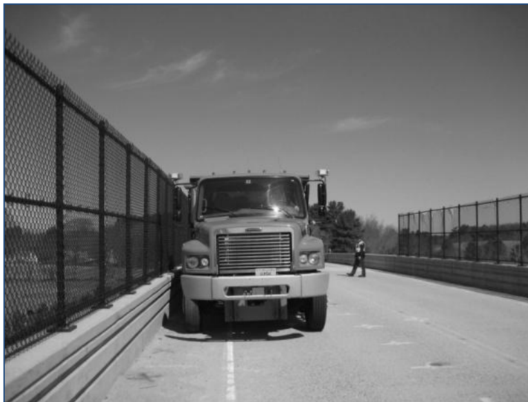
Figure 15: NHDOT sand truck as load application during April 2008 load test
