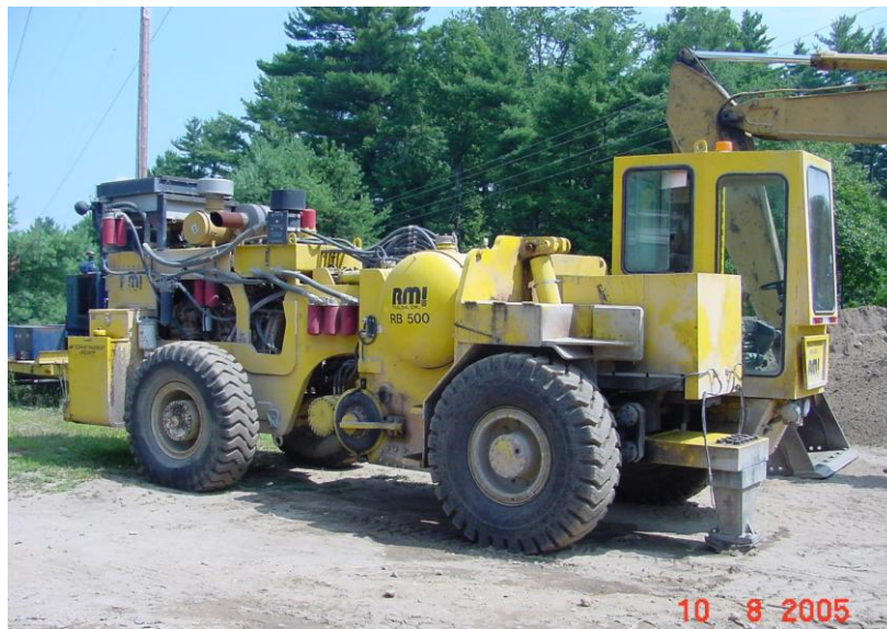
Figure 5 - Pavement breaker for rubblizing concrete
