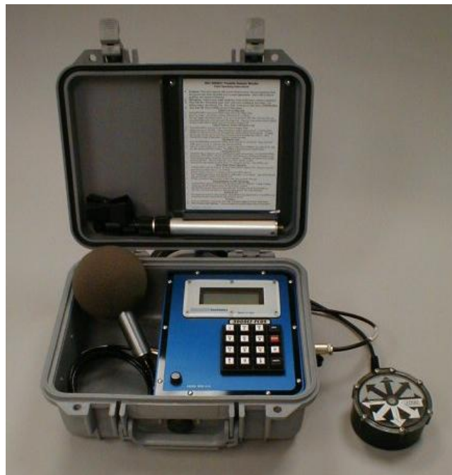
Figure 2 - GeoSonics SSU 3000 EZ Seismograph
