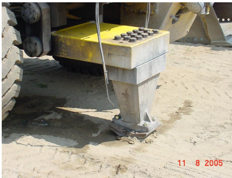
Figure 6 - Vibrating foot on pavement breaker
