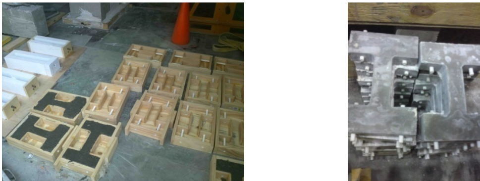
Figure 3.19 Fatigue Specimens during and after Casting
