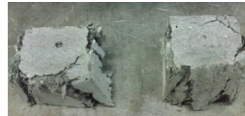
Figure 3.9 Block Batches after Failure
