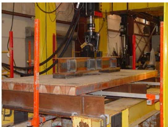
(a) (b) Figure 4.6 Test Setup: (a) Initial Static and Fatigue Tests and (b) Residual Strength Test
