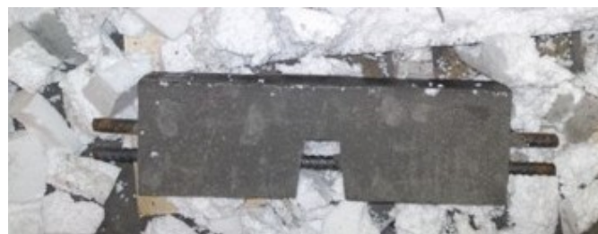
Figure 3.6 Actual Cast Dowel Action Specimen
