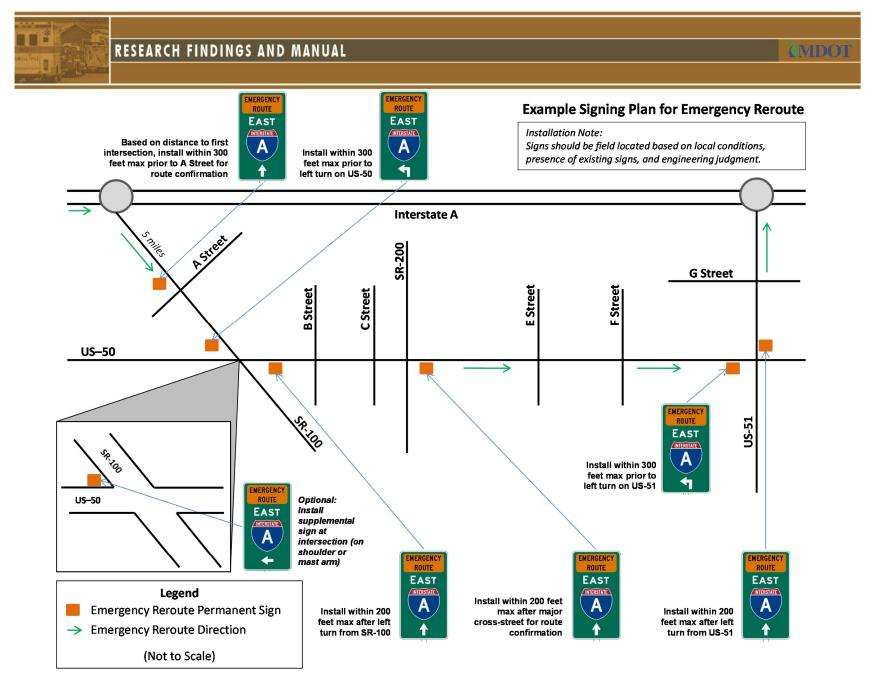
Figure 8. Example Signing Plan for Emergency Reroute
