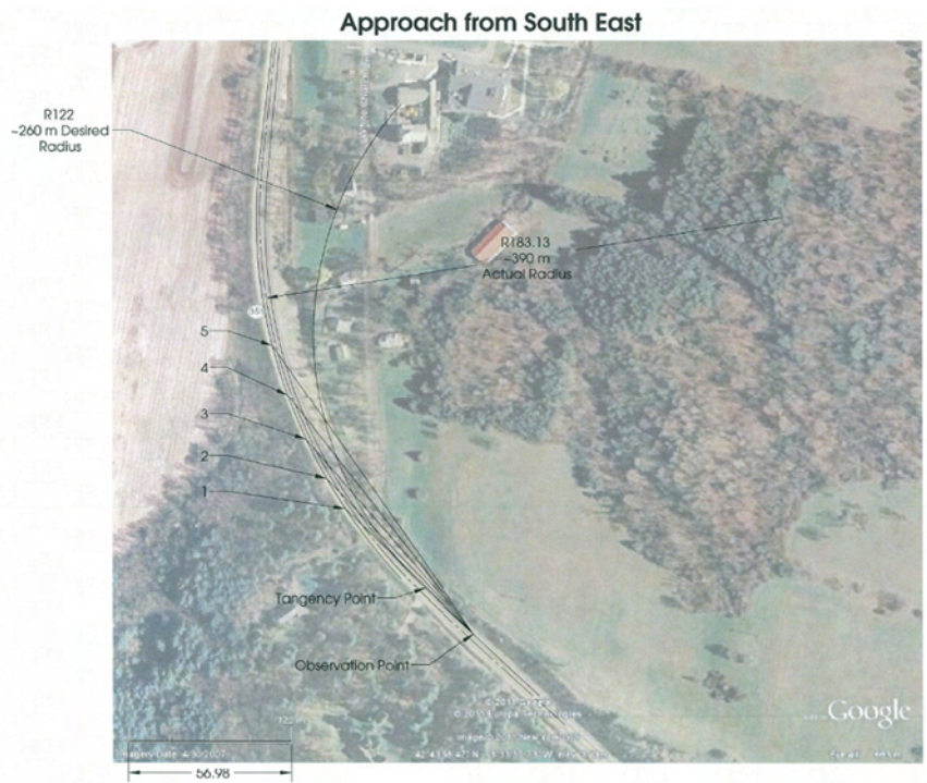
Figure 3-1. Proposed chevron locations as viewed by traffic approaching from the south along Route 351. The sizes of the chevron panels at each location (1-5) are as follows: 1) 24 by 30 inches, 2) 26 by 32 inches, 3) 27 by 33 inches, 4) 28 by 34 inches, 5) 30 by 36 inches.
