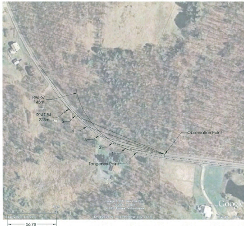
Figure 3-2. Proposed chevron locations as viewed by traffic approaching from the east along Route 43. The sizes of the chevron panels at each location (1-5) are as follows: 1) 18 by 24 inches, 2) 18 by 24 inches, 3) 20 by 26 inches, 4) 22 by 28 inches, 5) 25 by 31 inches. Following the installation of these signs, an additional 18 by 24 inch chevron panel was installed 20 m ahead of location #1, near the tangency point of the curve.
