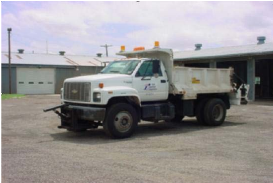
Figure 7-1. Dump Trucks Are the Workhorses of TxDOT Snow Removal.
