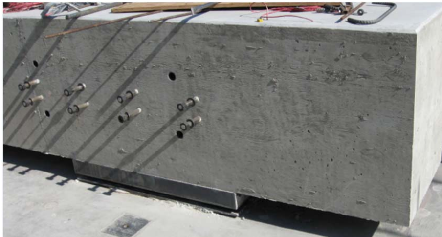
Figure 8.23 Roller Sandwich Assembly - Three Pile Specimen
