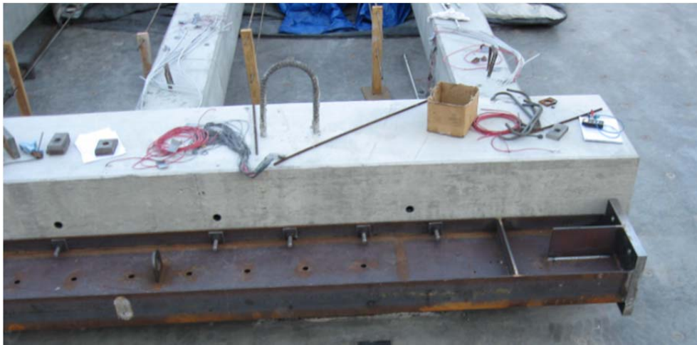
Figure 8.27 Loading Assembly - Three Pile Specimen
