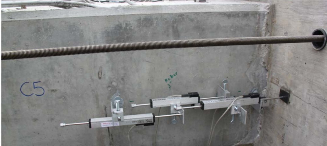
Figure 8.30 Novatecknic Gages - Three Pile Specimen
