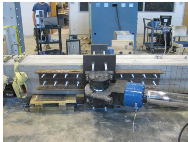
Figure 4.11 Actuator Connection at Pile - Exterior Specimens
