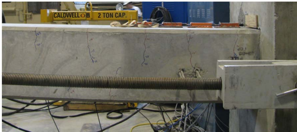
Figure 6.26 Observed Pile Curvature - Specimen IB-26-1
