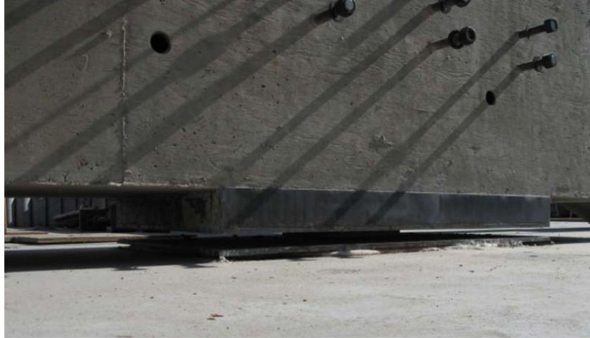
Figure 8.24 Roller Sandwich Assembly - Three Pile Specimen
