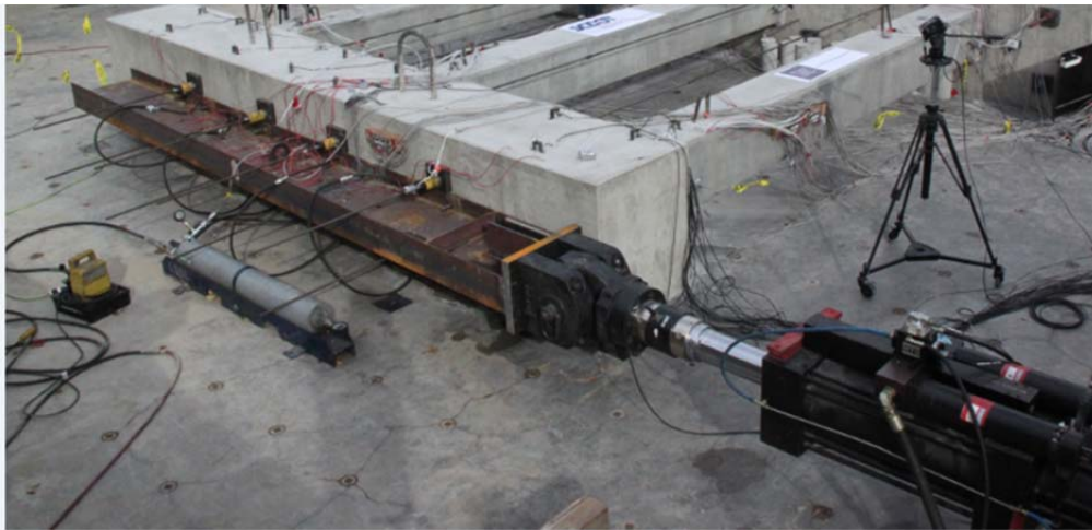
Figure 8.29 Loading Assembly - Three Pile Specimen
