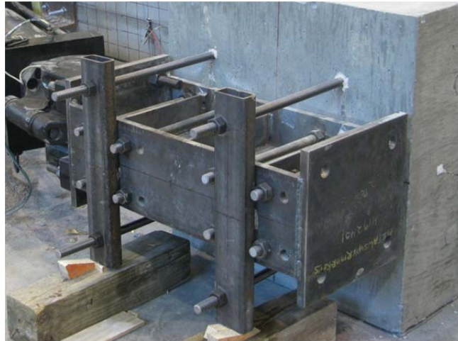
Figure 4.10 Actuator Connection at Bent Cap - Exterior Specimens
