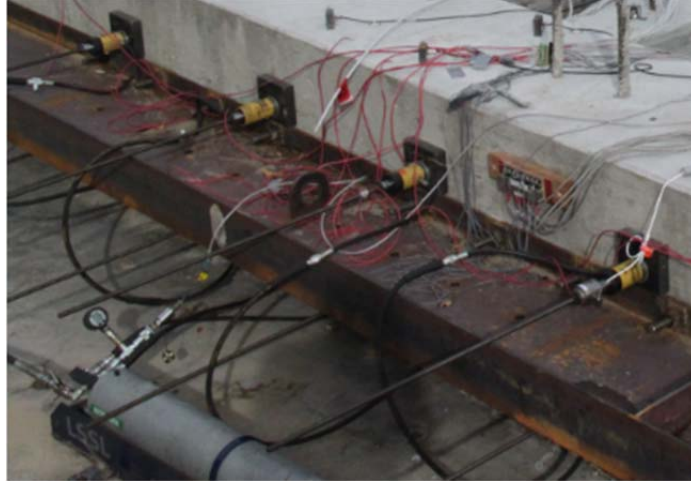
Figure 8.26 Axial Loading Setup - Three Pile Specimen
