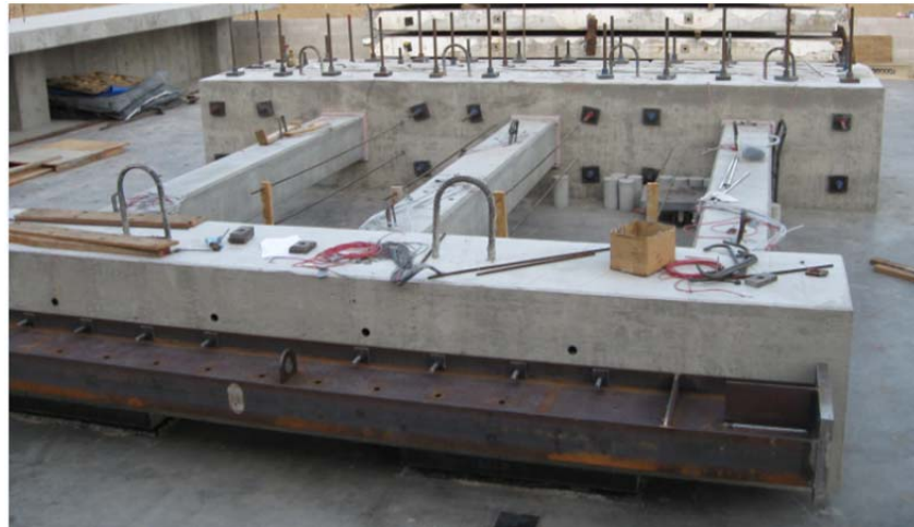
Figure 8.21 Testing Orientation - Three Pile Specimen
