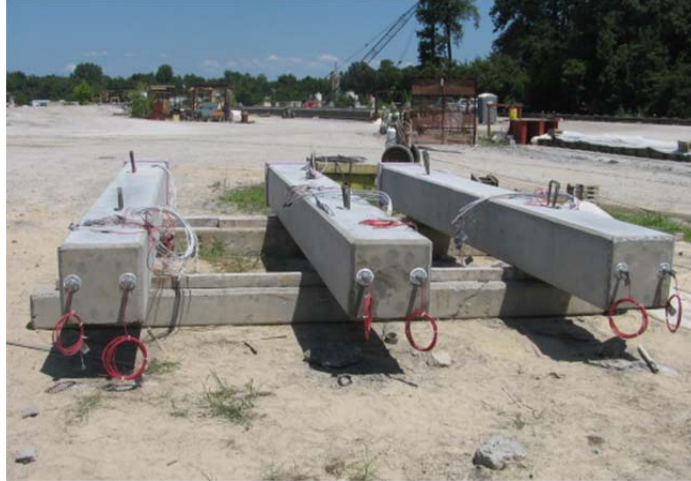
Figure 8.20 Linear Potentiometer Placement - Three Pile Specimen
