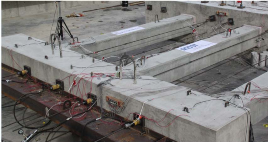
Figure 8.25 Axial Loading Setup - Three Pile Specimen
