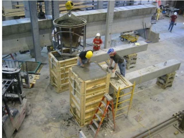
Figure 3.1 Casting of Bent Caps - Specimens IB-18-1 and EB-18-1
