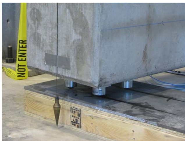
Figure 4.13 Four Roller End Support - Exterior Specimens
