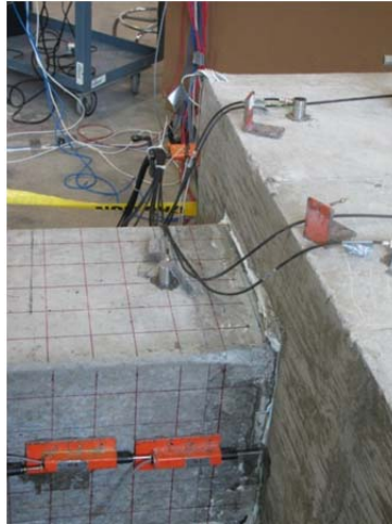
Figure 7.13 Pile Damage - Specimen EB-2-1
