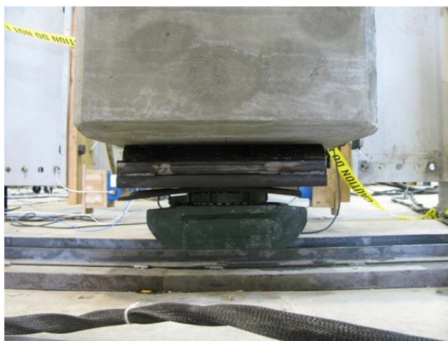
Figure 4.12 Hillman Roller End Pile Support - Exterior Specimens
