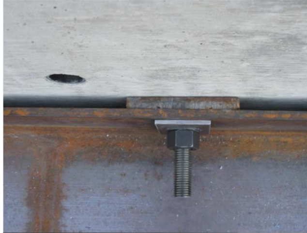
Figure 8.28 Transfer Beam Connection - Three Pile Specimen
