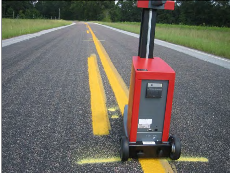
Figure 3.4: Retroreflectometer Collecting Data
