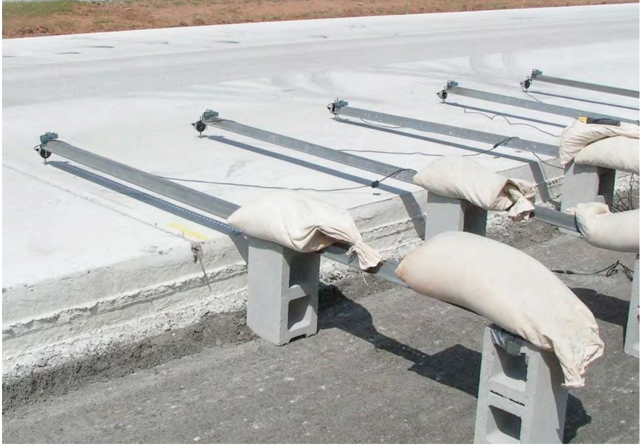
Figure 1 Set-up of digital indicators at I-385 test site.
