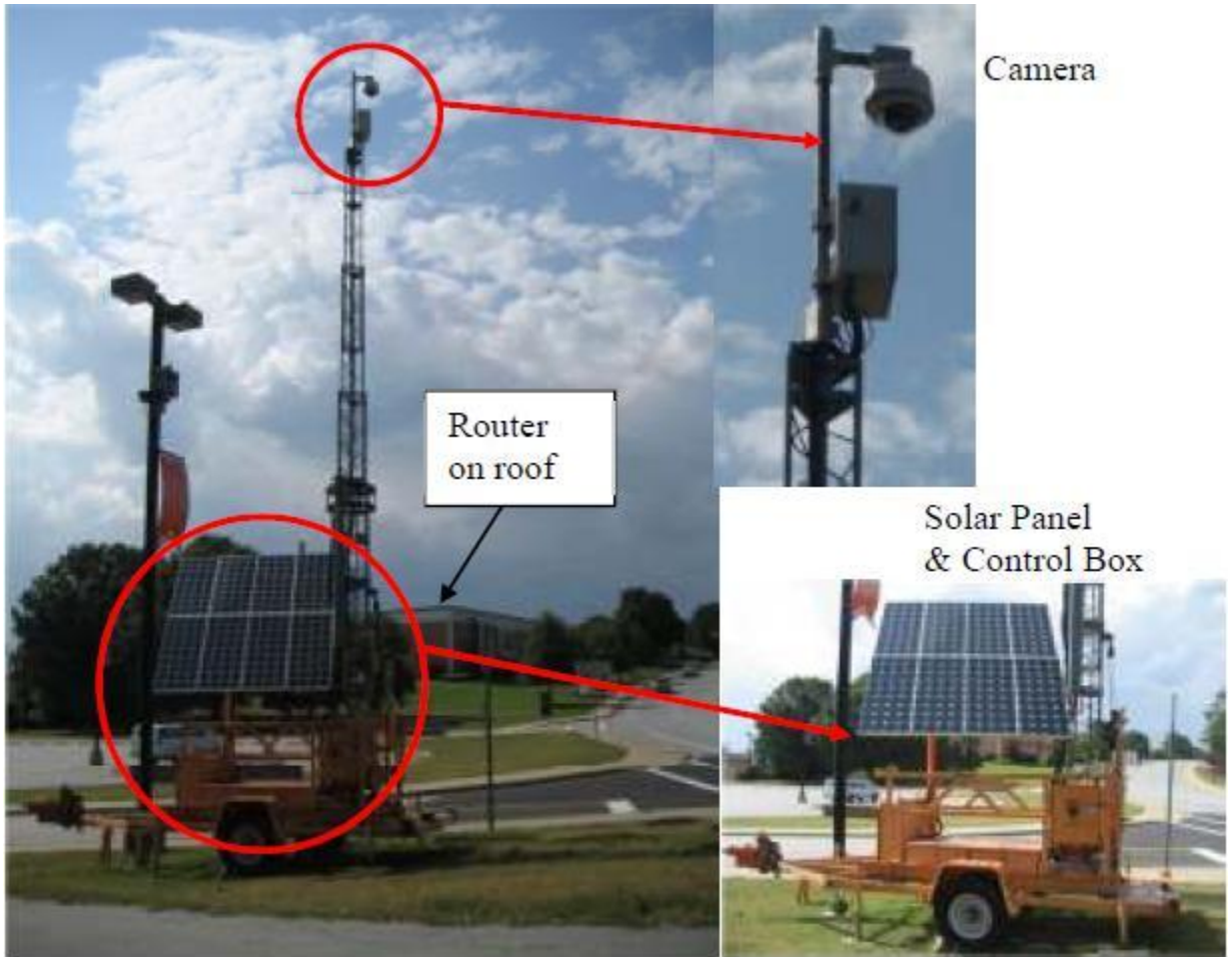
Figure 22 Solar power supported mobile traffic camera
