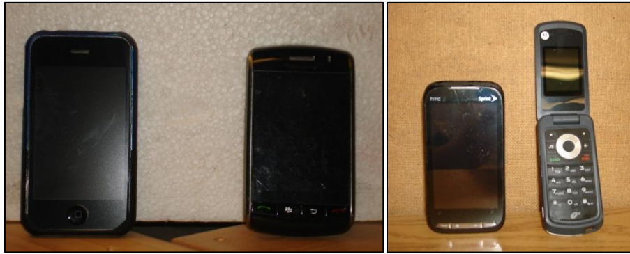
FIGURE 1 Bluetooth Enabled Cell Phones Used for Comparison Testing, Left to Right: Apple iPhone 3GS, Blackberry Storm, HTC Touch Pro2, the Standard Testing Phone Motorola 408g
