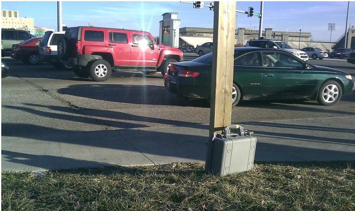
FIGURE 21 Bluetooth Data Logger Placement at Providence Road and Stadium Boulevard Intersection
