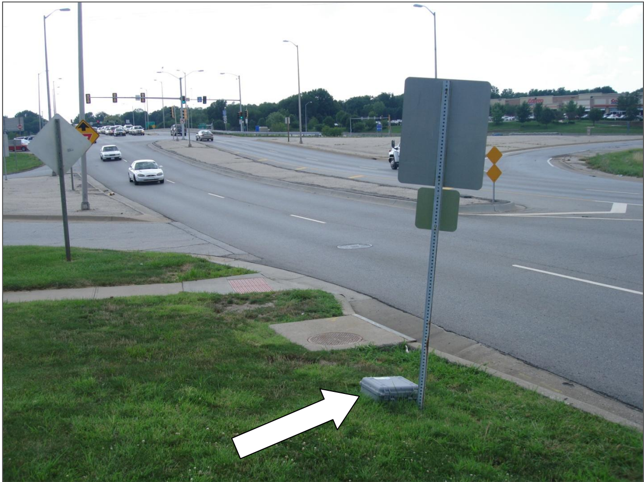
FIGURE16 Bluetooth Data Logger at the Northwest Corner of I-35 and 95th Street in Lenexa, Kansas
