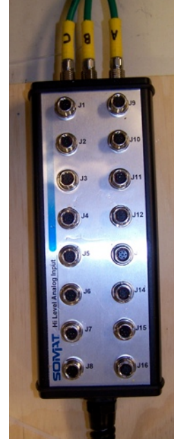
Figure 2.15 - Diagram and photograph of SoMat Connector Box and channel designations
