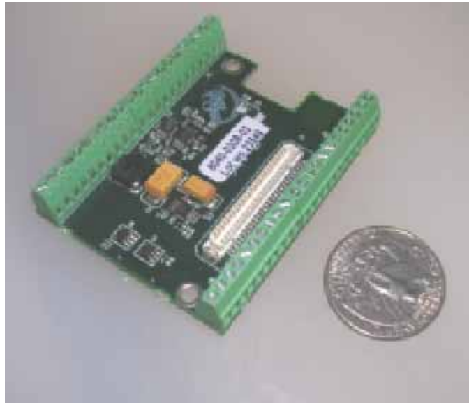
Figure 3.6: Photograph of a Crossbow MDA300 with quarter for scale, after Dowding et al. (2007)
