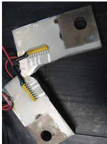
Figure 4.21: Coupon with custom gage after all rungs broken
