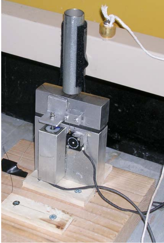
FIG. 3 A test mechanism to measure the transient response with LVDT (on the right) and potentiometer sensors (on the left)
