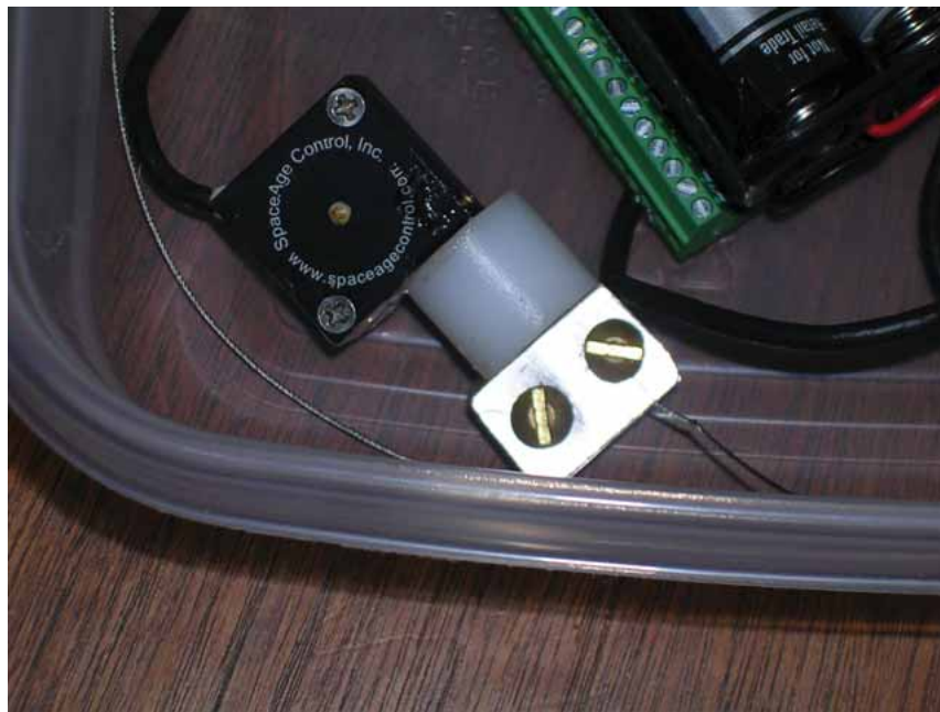
Figure 3.15: A string potentiometer measuring the expansion and contraction of a plastic donut
