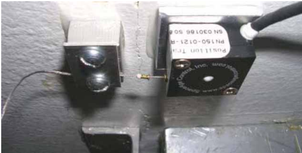
Figure 3.3: Photograph of a fully mounted string potentiometer, after Ozer (2005)
