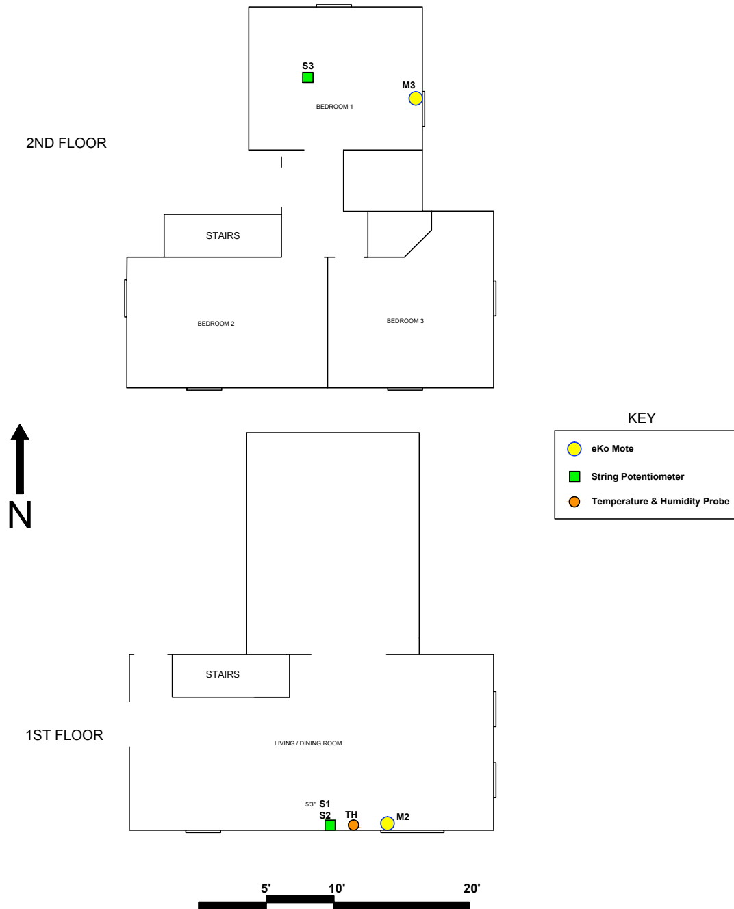
Figure 2.7 - Exact sensor and equipment locations within house. Measure given is distance up wall
