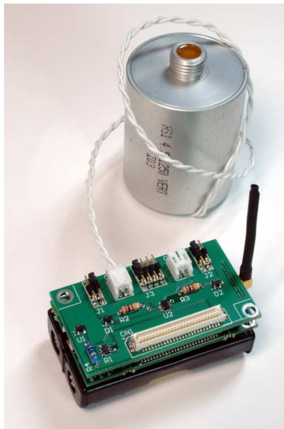
Fig. 1. Geophone connected to Mote-Wake board mated to Crossbow mote.
