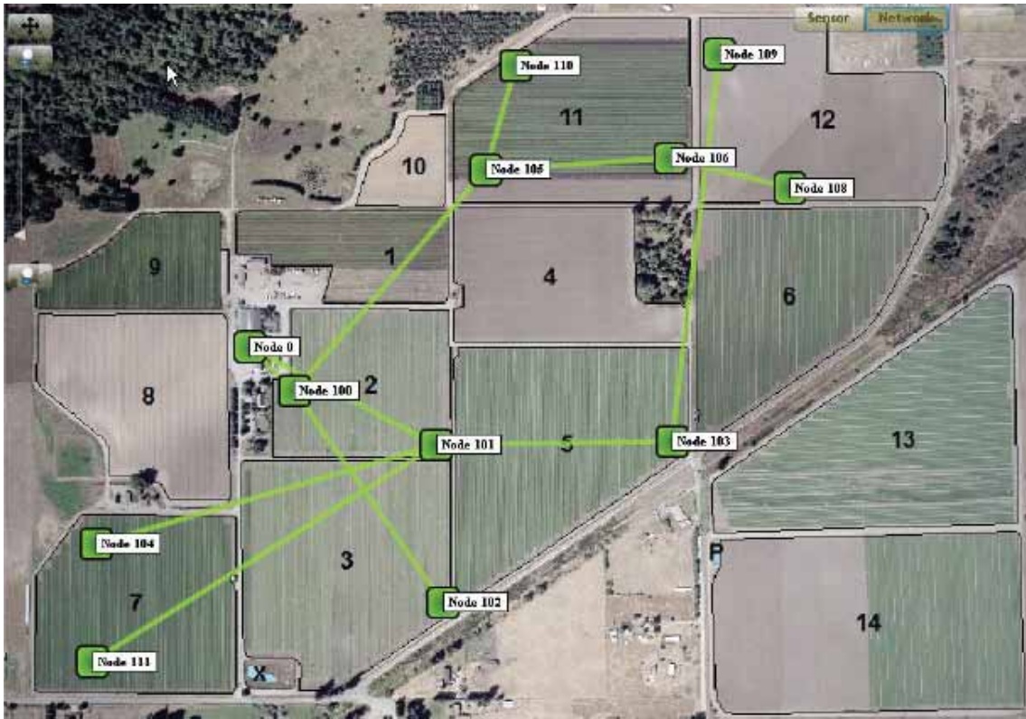
Figure 3.1: Example of a multi-hop network: green lines represent reliable radio links between motes, after Crossbow Technology, Inc. (2009b)
