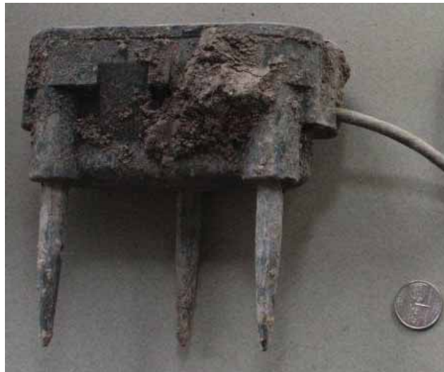
Figure 2.6: Photograph of a triaxial geophone with quarter for scale
