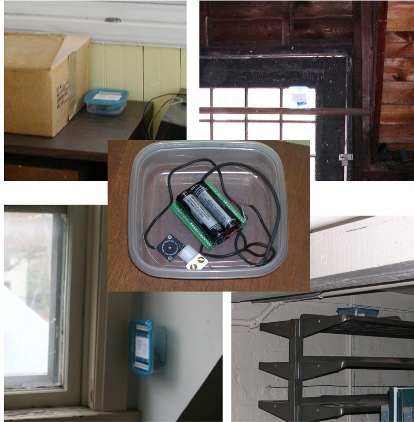
FIG. 5: Collage of photographs of the mote nodes in place that demonstrates their small size and multiple modes of placement. Clockwise from upper left: Sun porch, garage, basement, and apartment. Center photograph is that of the node with the same potentiometric displacement sensor shown in Fig. 2.
