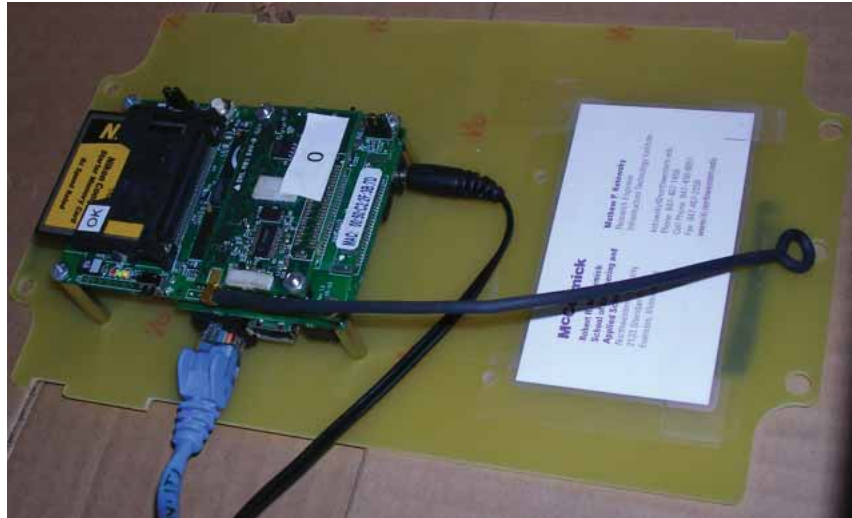
Figure 3.10: The Stargate Gateway mounted to a plastic board
