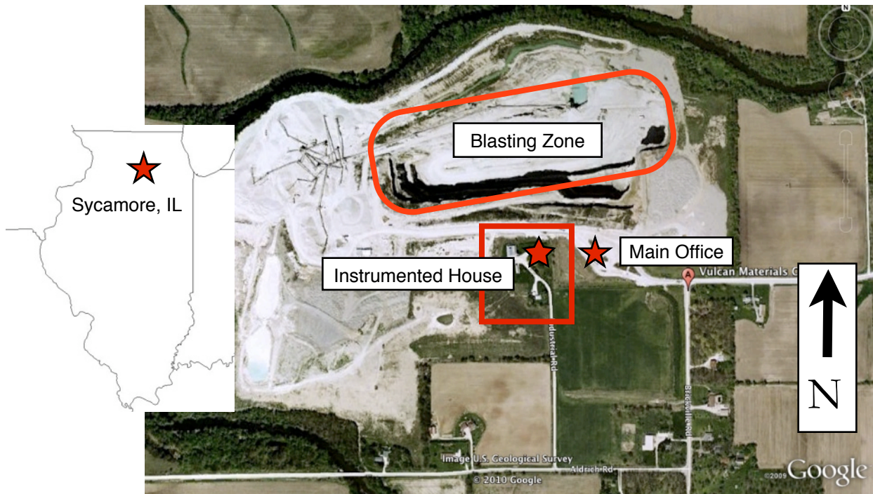
Figure 1.2 - Overall view of Vulcan Materials, Co. Sycamore Quarry #397 showing location of the Floit house in relation to the blasting zone
