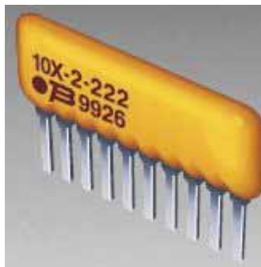
Figure 4.17: Photograph of a commercially available bus resistor, after Bourns (2006)
