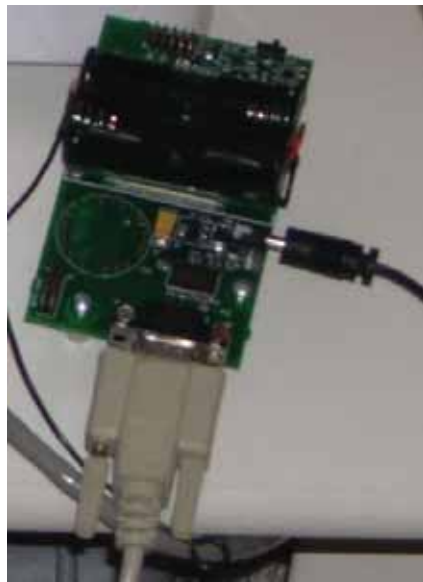
Figure 3.5: Photograph of a Crossbow MIB510CA serial gateway with MICA2 (without batteries) installed, after Ozer (2005)
