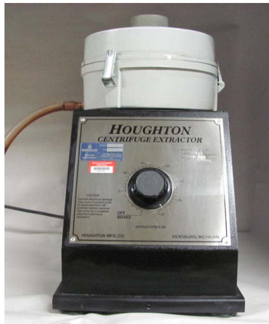
Figure 3-6. Centrifuge Used for Asphalt Extraction
