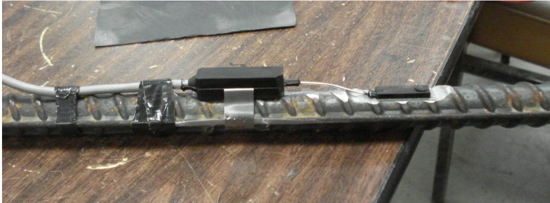
Figure 2.4: Strain gage after spot welding.
