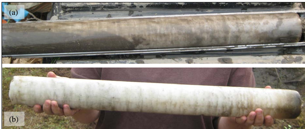
Figure 3.3. Split-spoon samples of massive ice, TH09-1401: a) ice with silt from 15.5-17.5 ft bgs; b) ice from 23.0-25.0 ft bgs.
