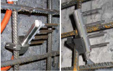
Concrete corrosion and Humidity sensors
