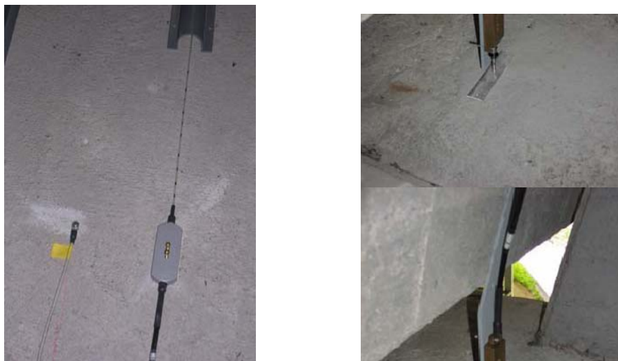
Fig. 21.26 Optical Sensors; Osmos Optical strand SI 5m (left) and Osmos EX 5mm (right)
