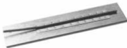
Fig. 4.11 A close-up view of a weldable FOS strain gauge
