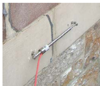
Fig. 11.2 Crackmeter unit shown with standard rebar anchors
