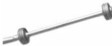
Fig. 4.10 A close-up view of an embeddable FOS strain gauge
