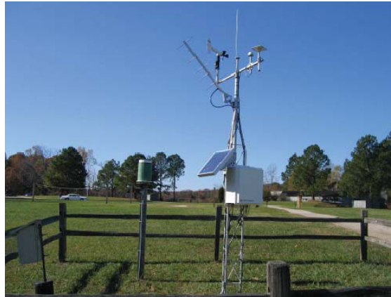
Fig. 16.3 This station for the National Estuarine Research Reserve (NERR) in Virginia transmits data via CSI GOES satellite transmitter
