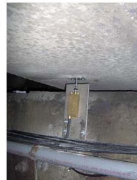
Fig. 12.3 Optical extensometer as a WIMS
