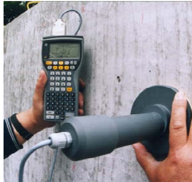
Fig. 18.2 GalvaPulse™: Hand held computer and electrode
