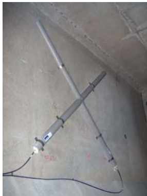
Fig. 13.7 Orthogonal Optical Strands to measure shear stress (Champlain Bridge, Montreal, Canada)
