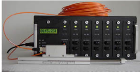
Fig. 16.8 A complete FOS system (Smart Structures, LLC)
