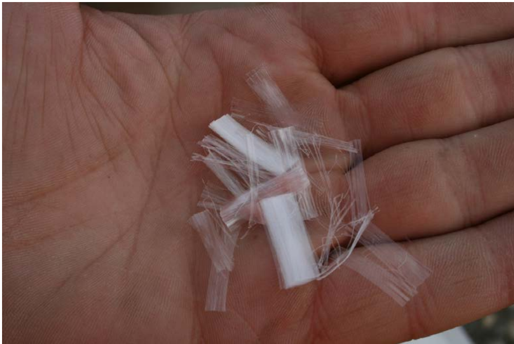
Figure 8: Fibers used on Horseshoe Lake road
