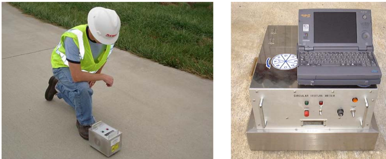
Figure 11. Commercially available laser based texture profilers. Left: Ames Engineering model 9200 Texture Scanner. Right: Nippo Sangyo Co., Ltd. Circular Track Meter (CTM).
