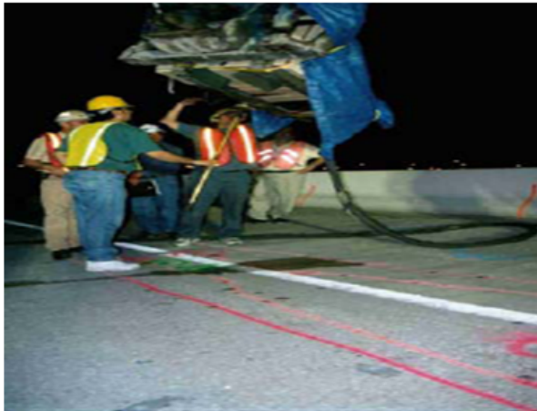
Figure A.13: X-Ray inspection of post-tensioned deck ramp D in Fort Lauderdale: x-ray inspection equipment (left) and example film radiograph (right) (DMJM Harris, 2003)
