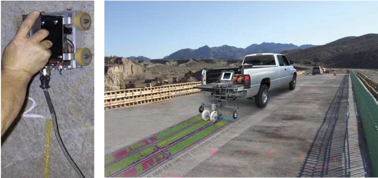
Figure A.16: Olson impact echo scanning equipment: handheld unit (left) and vehicle mounted unit (right)
