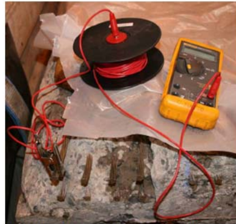
Electrical connection to strands
