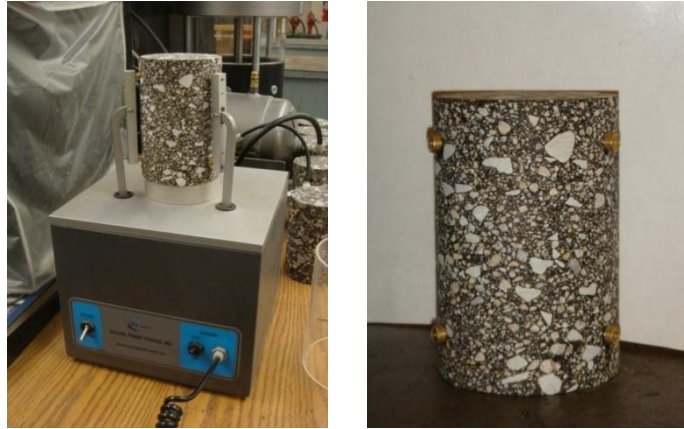
Figure 4.2 A device used to place the mounting studs for LVDTs
