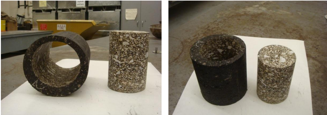
Figure 4.1 A specimen cored and sawn from the gyratory compacted sample
