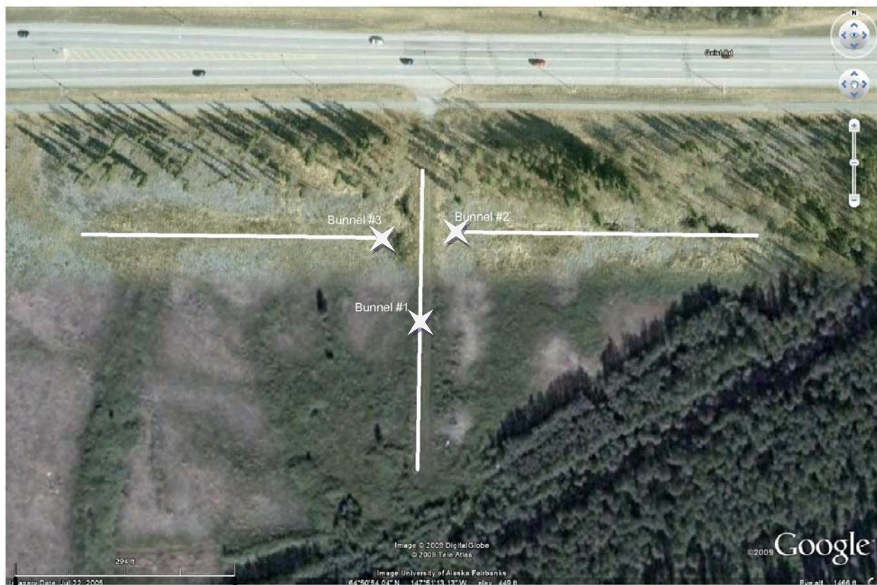
Figure 8 SASW array location map for Site 5 (Bunnel).
