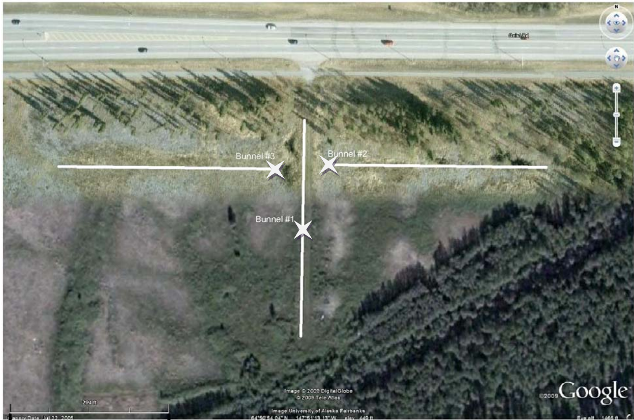
Figure 13 SASW Array location map for Site 5 (Bunnel).
