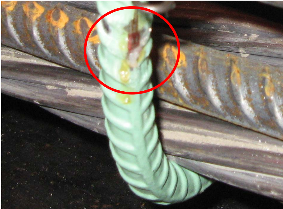
Figure 31 – Surface gage mounted on an epoxy coated bottom flange stirrup and silicone coating.
