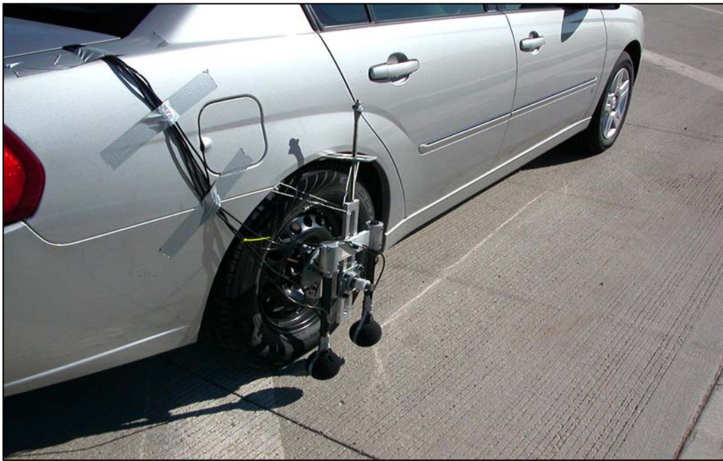
Figure 4: Dual probe OBSI fixture installed on car test with ADOT test tire in November 2006
