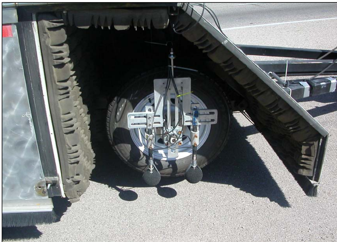
Figure 3: Dual probe OBSI fixture installed on the ADOT CPX trailer for comparative testing in March 2005.
