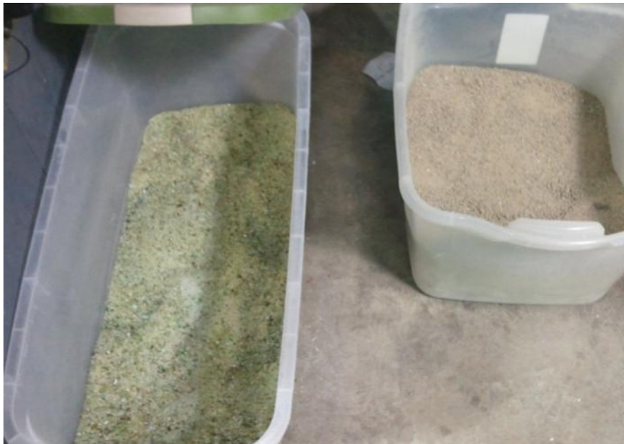
Figure 3-2: 3000 revolution glass sand (left) and natural river sand (right) as used in concrete production
