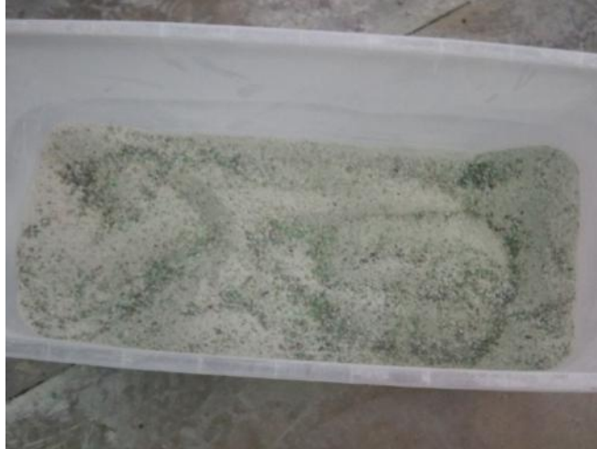
Figure 3-4: 1000 revolution glass sand used in production of concrete mixtures
