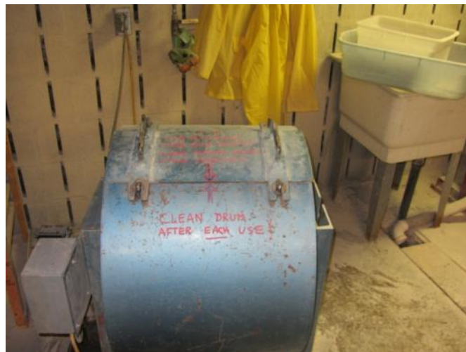
Figure 3-3: LA Abrasion Machine used to crush glass cullet to sand size
