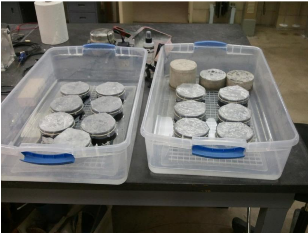
Figure 3-9: (Top) Schematics of a specimen's exposure to water during the sorptivity test; (bottom) Water bath setup in ASTM C1585
