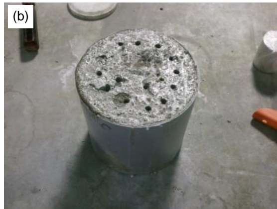
Figure 3-5: (a) Humboldt H/4133 spring-reaction device used for measurement of time of setting of mortar; (b) Mortar specimen after completion of setting time measurements
