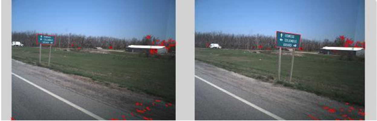
Figure 5.3: Two subsequent images obtained from the video log. The highlighted regions indicate the segments that remain after size and color based classification.
