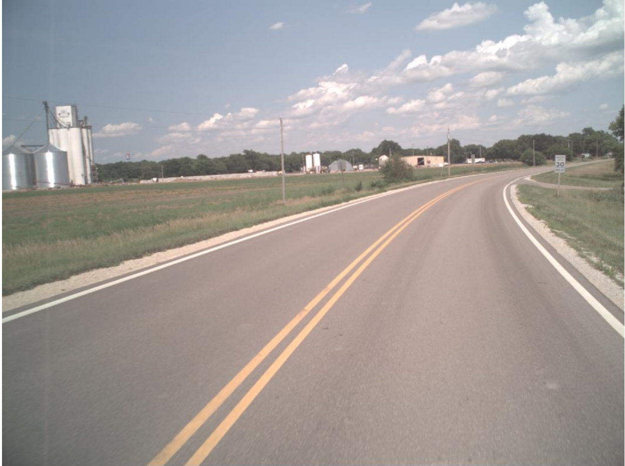
Figure 7.3: Usually images are taken with straight line motion between frames, and the vectors \vec{C}_1 and \vec{C}_2 are accurately known. However, on curved roads the straight line assumption is not met and triangulation error is high.
