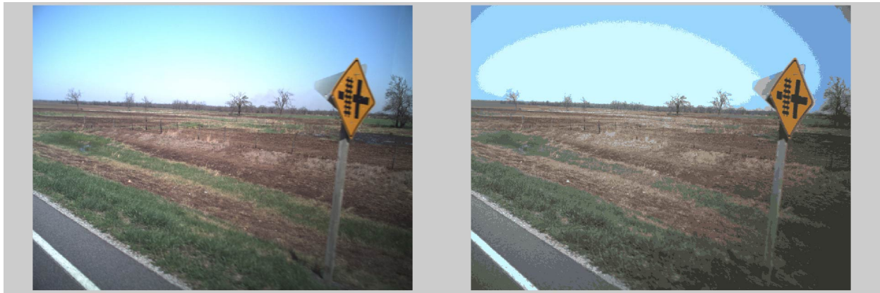
Figure 2.1: This figure shows the original image and the color segmented image obtained using K-Means Clustering on an image with a yellow road sign. In the color segmented image the pixels belonging to the yellow portion of the road sign are grouped into a segment.
