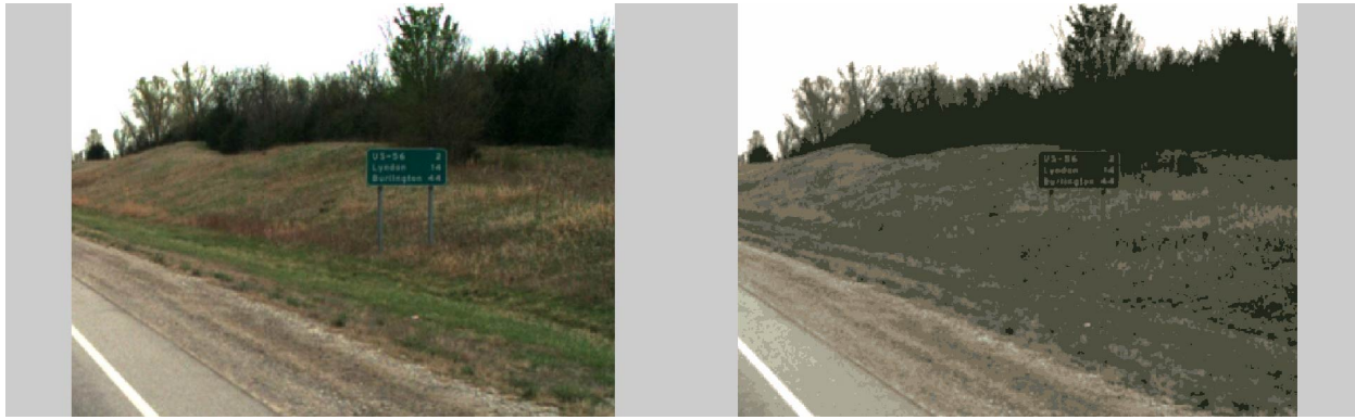
Figure 2.2: Here, the green sign's color is not one of the 16 color centers. Its pixels are shifted to the closest cluster center resulting in under segmentation.
