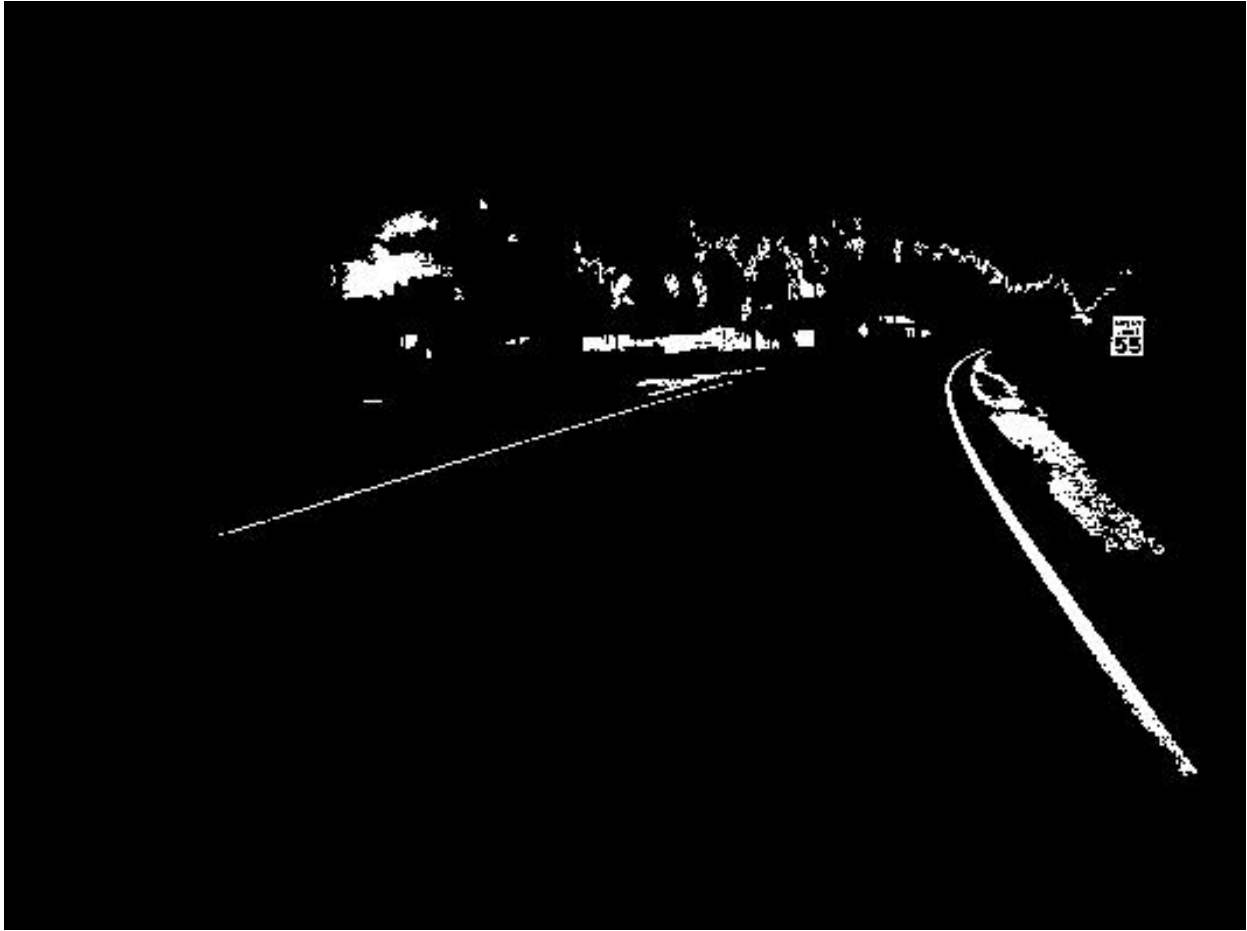
Figure 9.5: \alpha = 0.1, y_\eta obtained is 172. More false positives. All the segments that have pixels whose Red, Green and Blue values are above y_\eta are classified as white road signs.
