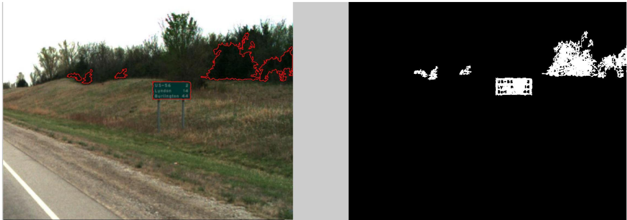
Figure 3.3: Results of color based classification on segments obtained in 3.1. The highlighted regions depict the segments with a color distribution similar to that of road signs.
