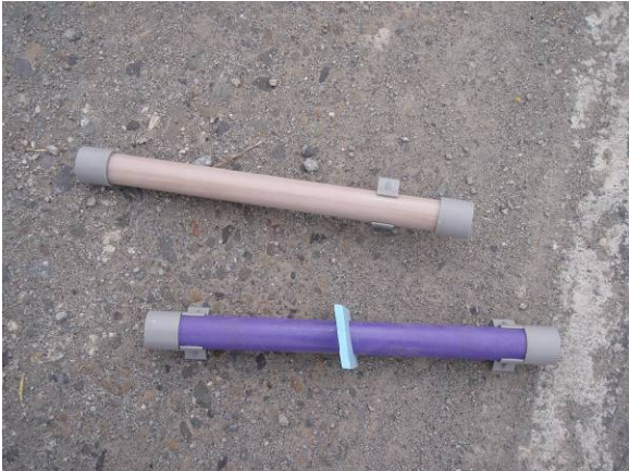
Figure 4. GFRP bar top, epoxy coated bar bottom.
