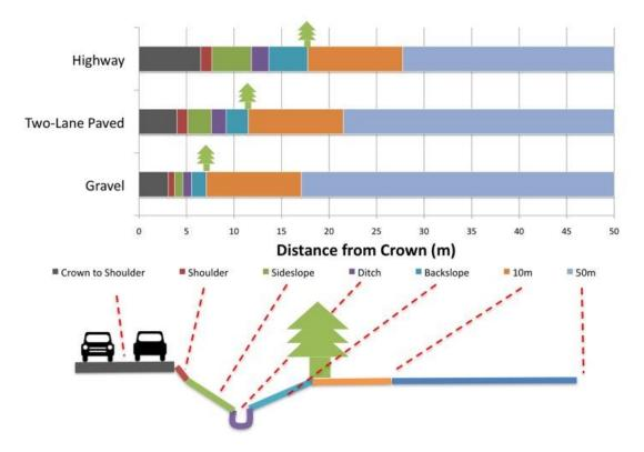
**Figure 2-3.** Measured Dimensions of Roadside Microtopography. Tree icon represents the edge of the forest which was defined as visually in line, and parallel the road, with he first tree > 8 cm diameter at breast height (DBH). The road crown (0m) is effectively the center of each road type.
