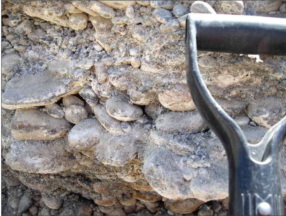
Figure 90. Pedogenically Formed Carbonate Coatings (Mixed with Opaline Material) in Duripan/Caliche Horizons at Ad-53s
