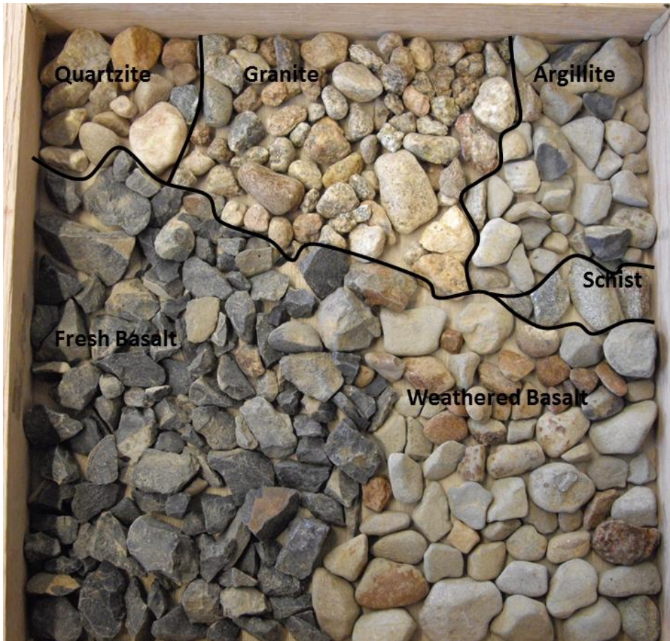
Figure 105. Vy-56c- ¾ Inch Aggregate
