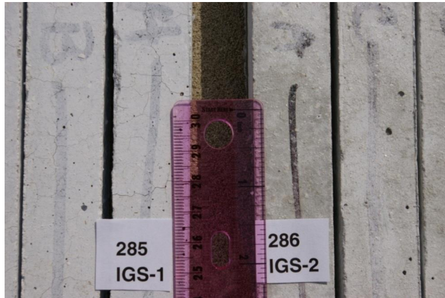
Figure 16. Mortar Bars IGS-1 and IGS-2 After AASHTO T 303 16-Day Expansion Test IGS-1 Illustrates a More Intense Pattern of Cracking than IGS-2
