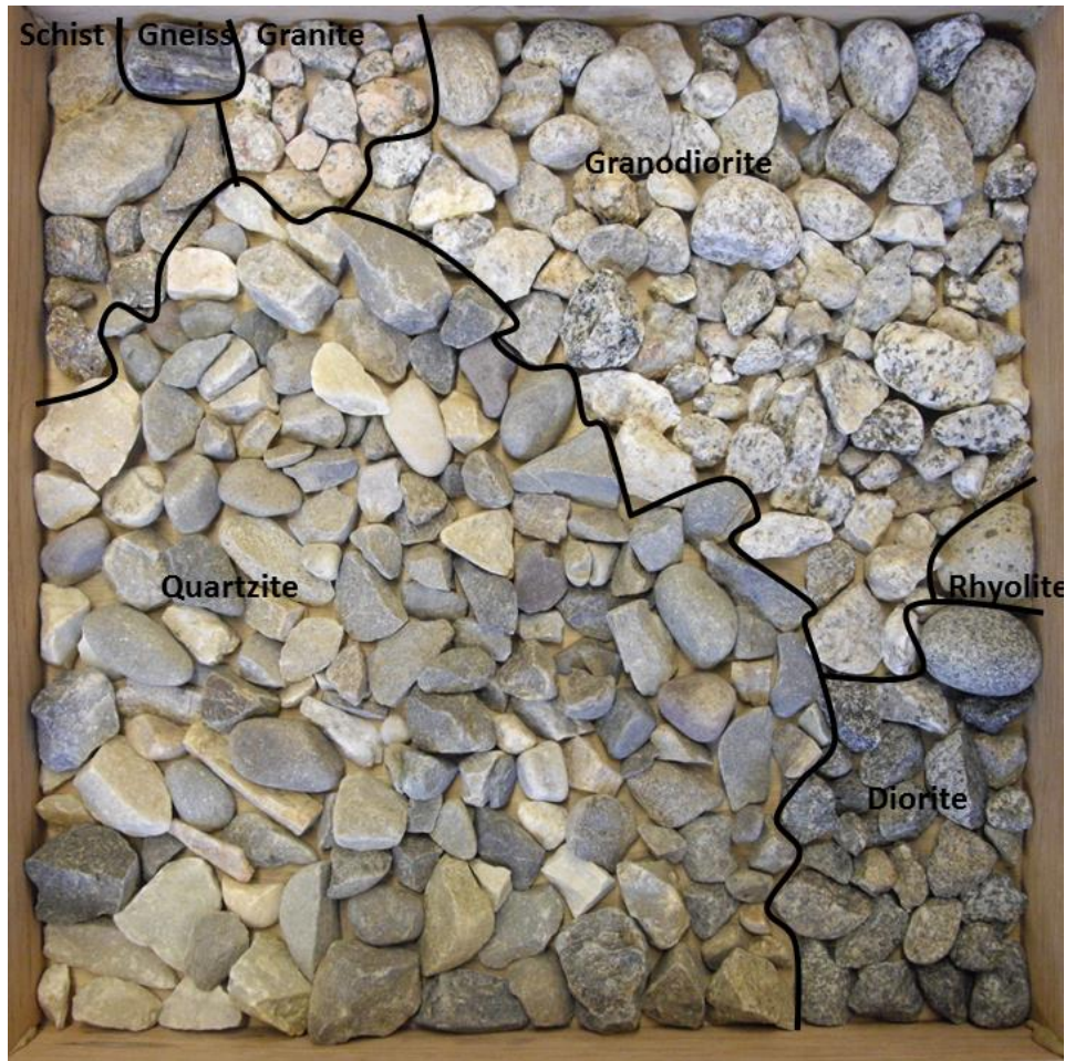
Figure 91. Br-2c - ¾ Inch Aggregate
