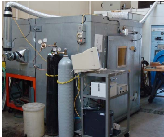
Figure 6: Chamber for hosting the pressure reactor unit.
