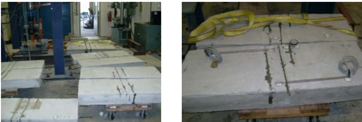
Figure 3-19: Sealed slabs with LVDT's and dial gages and sealed cracks
