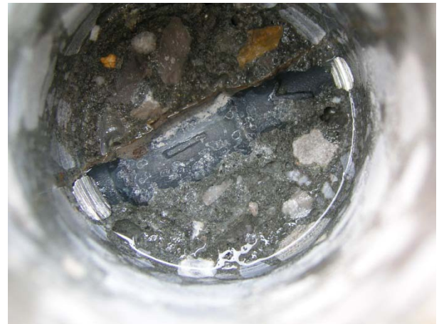
Figure 3-4: Core sampling showing crack development over the transverse reinforcement
