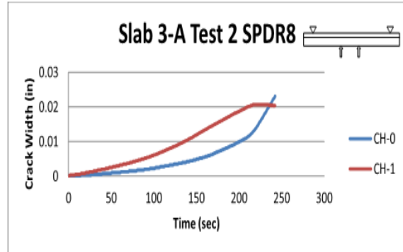
Figure 3-37: Slab 3-A crack width results
