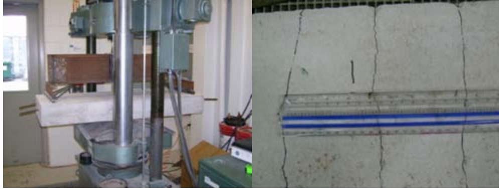
Figure 3-21: Testing of control slab specimen and crack development
