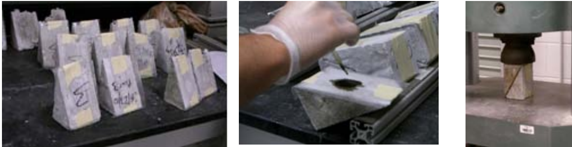
Figure 3-16: Applying the sealant to concrete specimens before and testing
