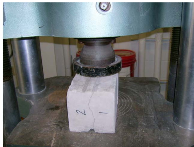
Figure 3-45: Beam during split test procedure
