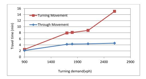
Figure 5-42 Effect of turning movement on through movement uncontrolled intersection in DynusT
