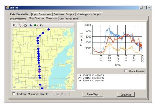
Figure 6-5 Variations of measures by time of day at each individual detector point
