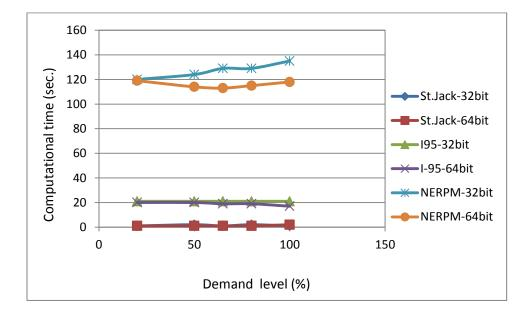
Figure 5-1 Computational time when utilizing Cube Voyager static assignment
