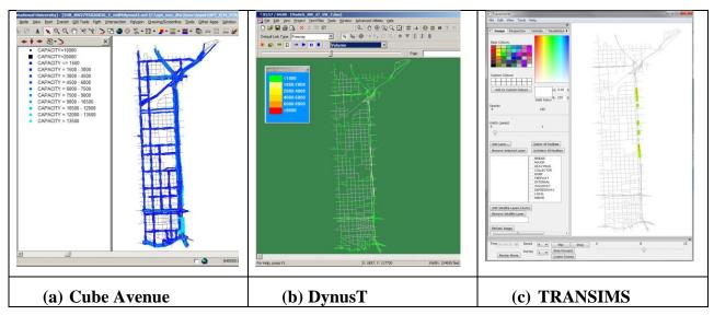
Figure 5-12 Visualizations of link performance in DTA tools
