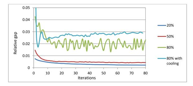
Figure 5-27 DynusT Gap-based method convergence for the I-95 network
