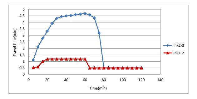
Figure 5-38 Demonstration of DynusT queue spillback (travel time over time)
