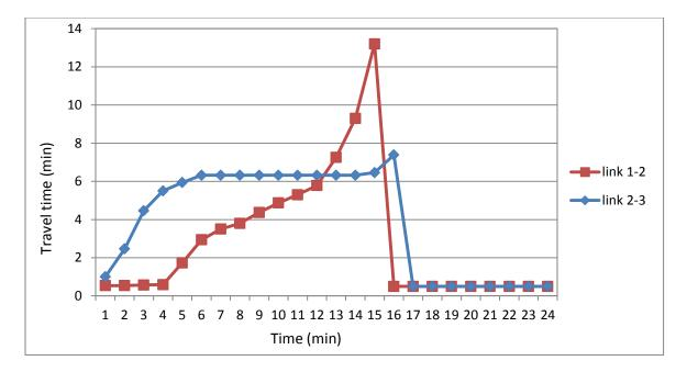
Figure 5-37 Demonstration of Avenue queue spillback (travel time over time)
