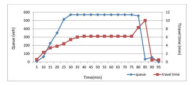
Figure 5-34 Avenue queue and travel time trend over time (jam density=120 veh/mile/ln)
