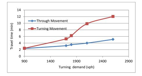
Figure 5-43 Effect of turning movement on through movement uncontrolled intersection in TRANSIMS
