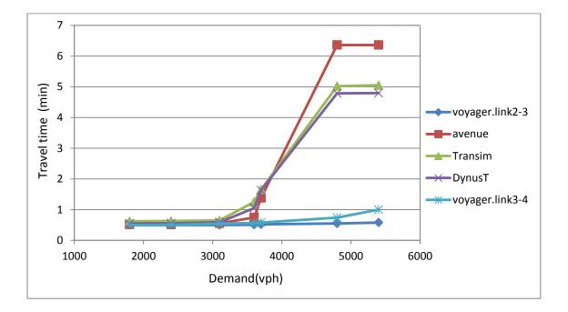
Figure 5-32 Demand-travel time relationships with capacity constraint from downstream link
