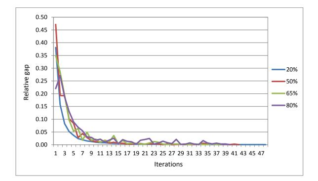
Figure 5-20 Cube Avenue PS method convergence for the I-95 network
