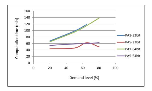
Figure 5-5 Computational time when utilizing Cube Avenue for the I-95 Network for PA packet size 1 and 5
