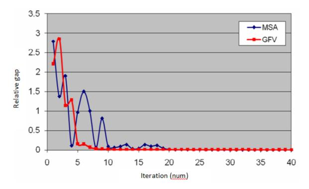
Figure 2-2 Comparison of MSA and GFV Assignment Method Convergence (Chiu and Bustillos, 2009)
