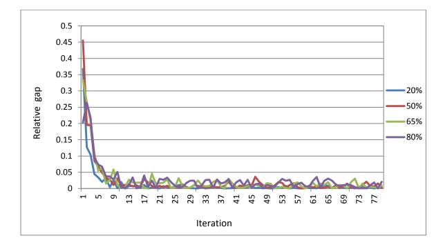
Figure 5-19 Cube Avenue PA method convergence for the I-95 network
