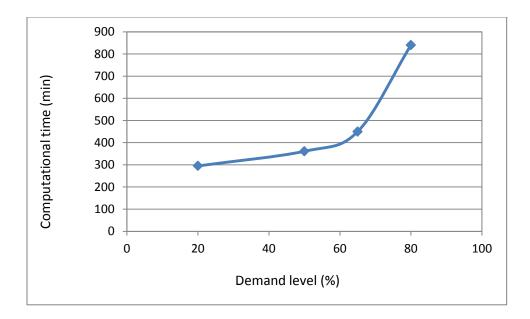
Figure 5-4 Computational time when utilizing Cube Avenue for the I-95 Network for PS
