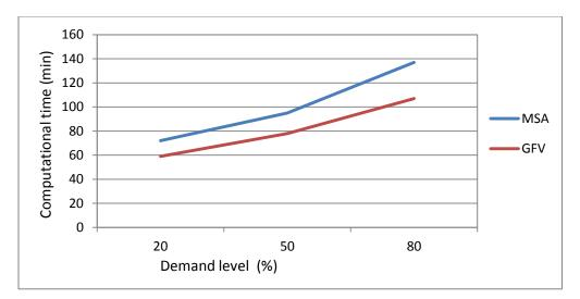
Figure 5-8 Computational time when utilizing DynusT with MSA and GFV Methods utilizing 64 bit Computer for Statewide Jacksonville
