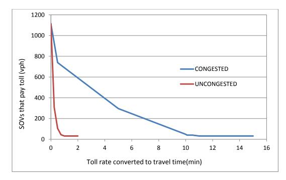
Figure 5-15 Cube Avenue dynamic assignment sensitivity to toll specification
