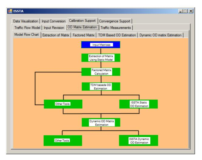
**Figure 6-10 O-D matrix estimation flow chart**
