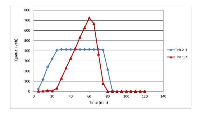
Figure 5-36 Demonstration of Avenue queue spillback (queue forming over time)
