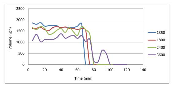
Figure 5-45 Variations in mainline volume with the increase in off-ramp volumes in DynusT
