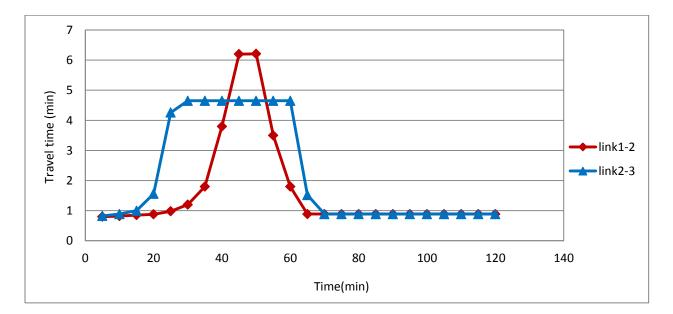
Figure 5-40 Demonstration of TRANSIMS queue spillback (travel time over time)
