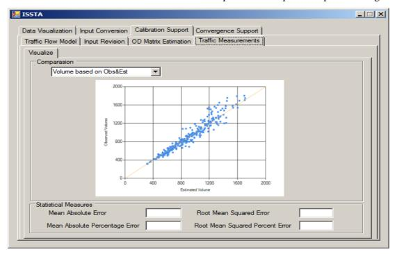
Figure 6-14 The traffic measurements user interface for comparison of observed and simulated volume comparison
