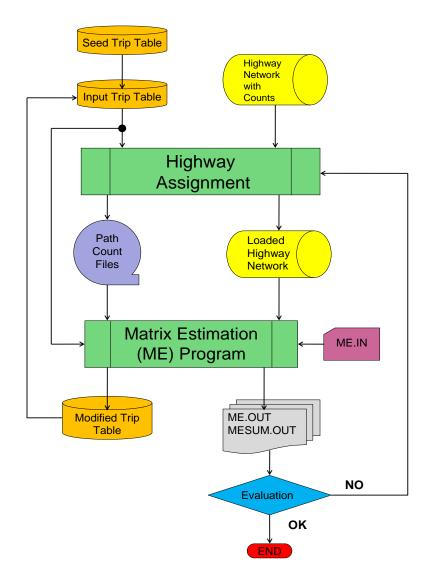
Figure 6-12 Static O-D estimation procedure
