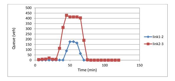
Figure 5-47 Avenue modeling of incident effects (jam density=295 veh/mile/ln)
