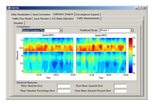
Figure 6-15 Example of speed counter plot comparison between real-world and observed speed counters output by ISSTA
