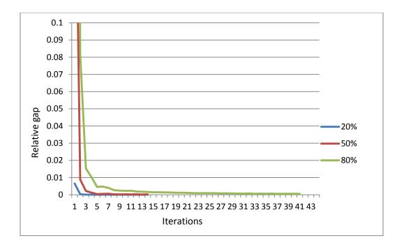
Figure 5-17 Cube Voyager, Network 2 (Statewide Jacksonville), relative gap vs. iteration
