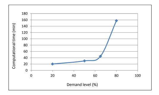
Figure 5-3 Computational time when utilizing Cube Avenue for the Statewide Model Jacksonville Network for PS mode
