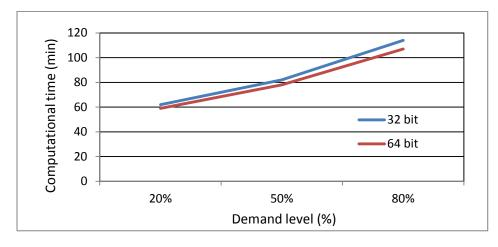
Figure 5-6 Computational time when utilizing DynusT with 32 and 64 bit computers for Statewide Jacksonville
