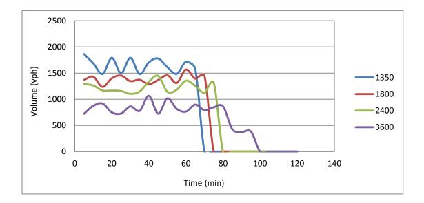
Figure 5-46 Variations in mainline volume with the increase in off-ramp volumes in TRANSIMS
