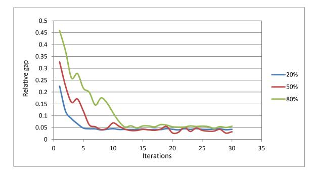
Figure 5-29 Convergence of DynusT Gap-based method for Statewide Jacksonville network
