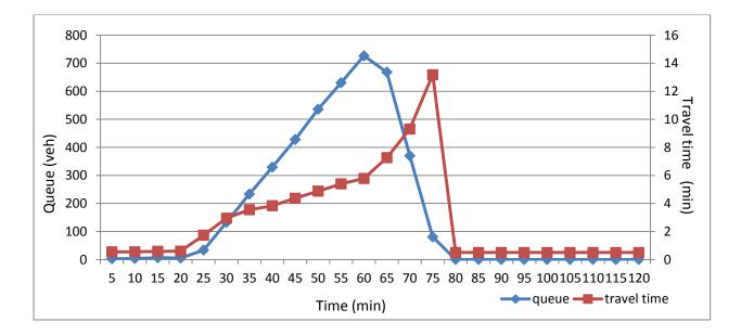
Figure 5-33 Cube Avenue queue and travel time trend over time (jam density=295 veh/mile/ln)
