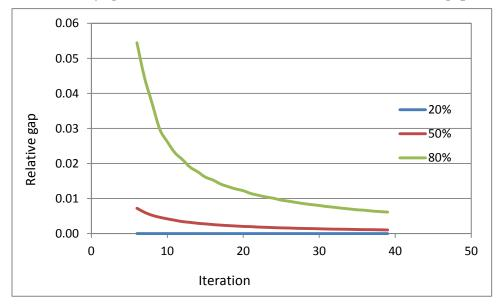
Figure 5-18 Cube Voyager convergence for NERPM Jacksonville network for different demand levels.
