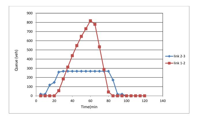
Figure 5-39 Demonstration of TRANSIMS queue spillback (queue over time)
