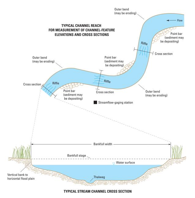
Figure 2. Typical channel reach and cross section for measurement of channel features.
