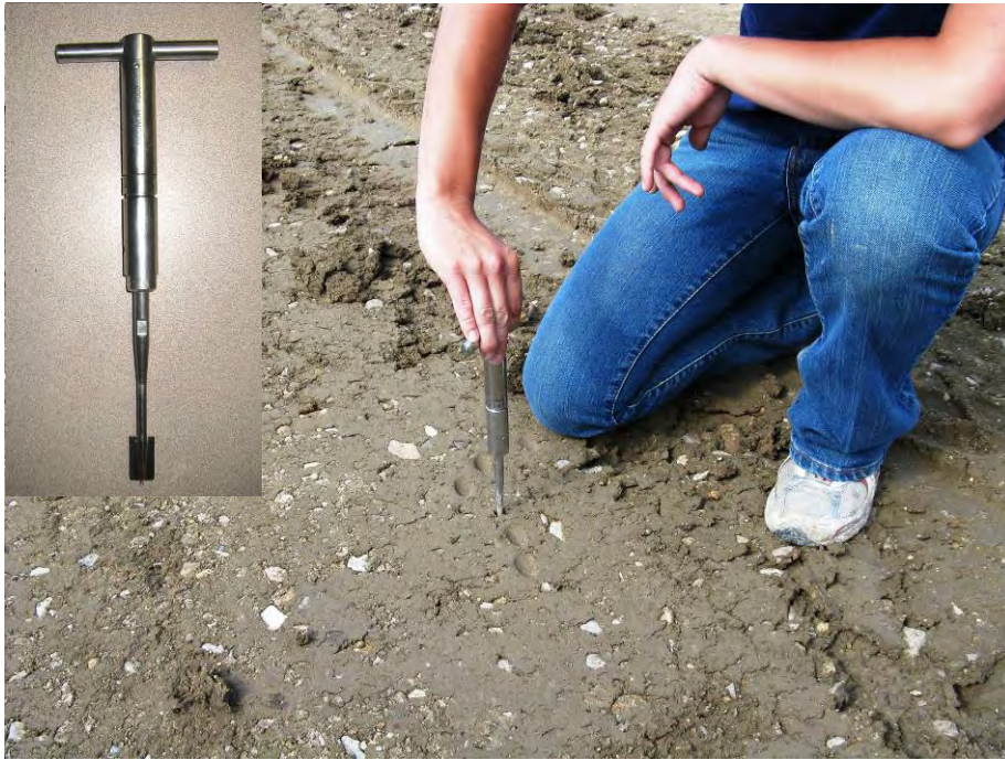
Figure 18. Field measurement of vane shear (inset is close-up of vane shear device).
