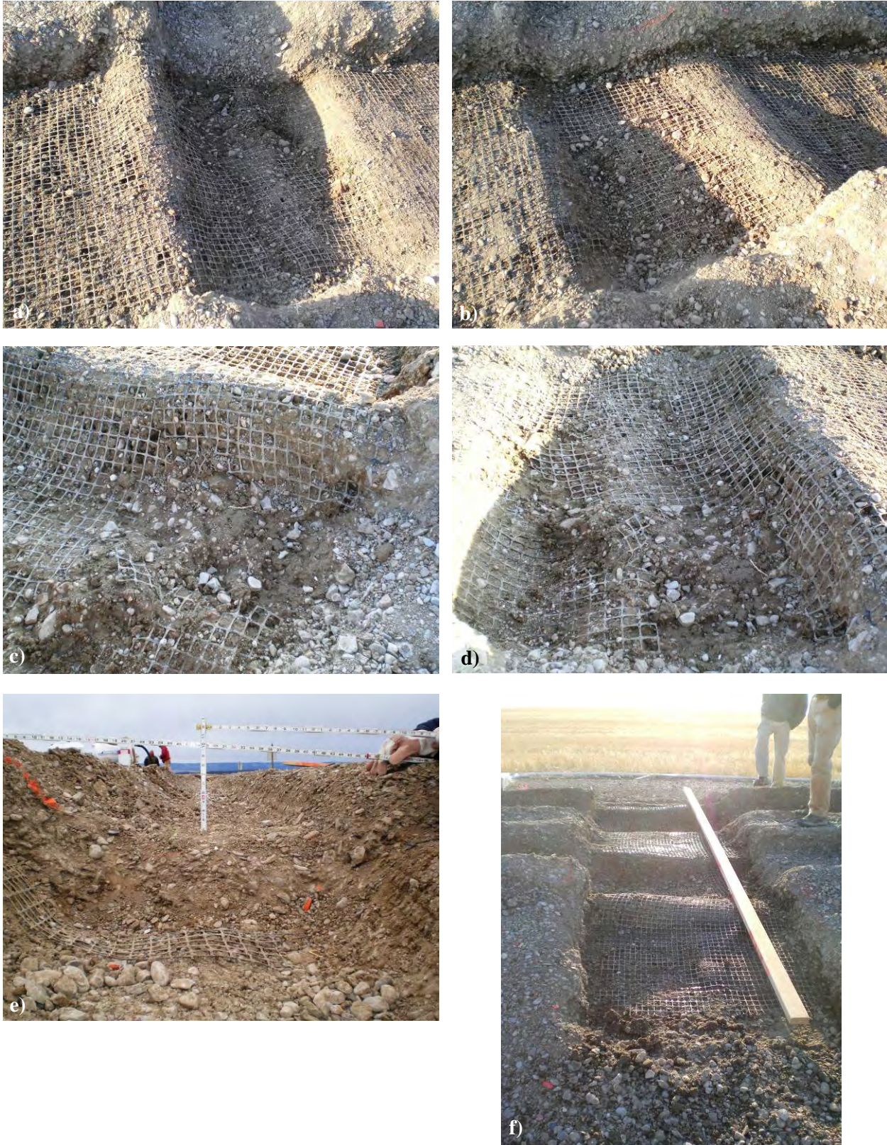
Figure C-14. Photos of the forensic excavations of the IFG-3 test section: a) rut bowl, b) rut bowl, c) close-up of side of rut bowl, d) close-up of rut, e) rut profile and f) looking west.
