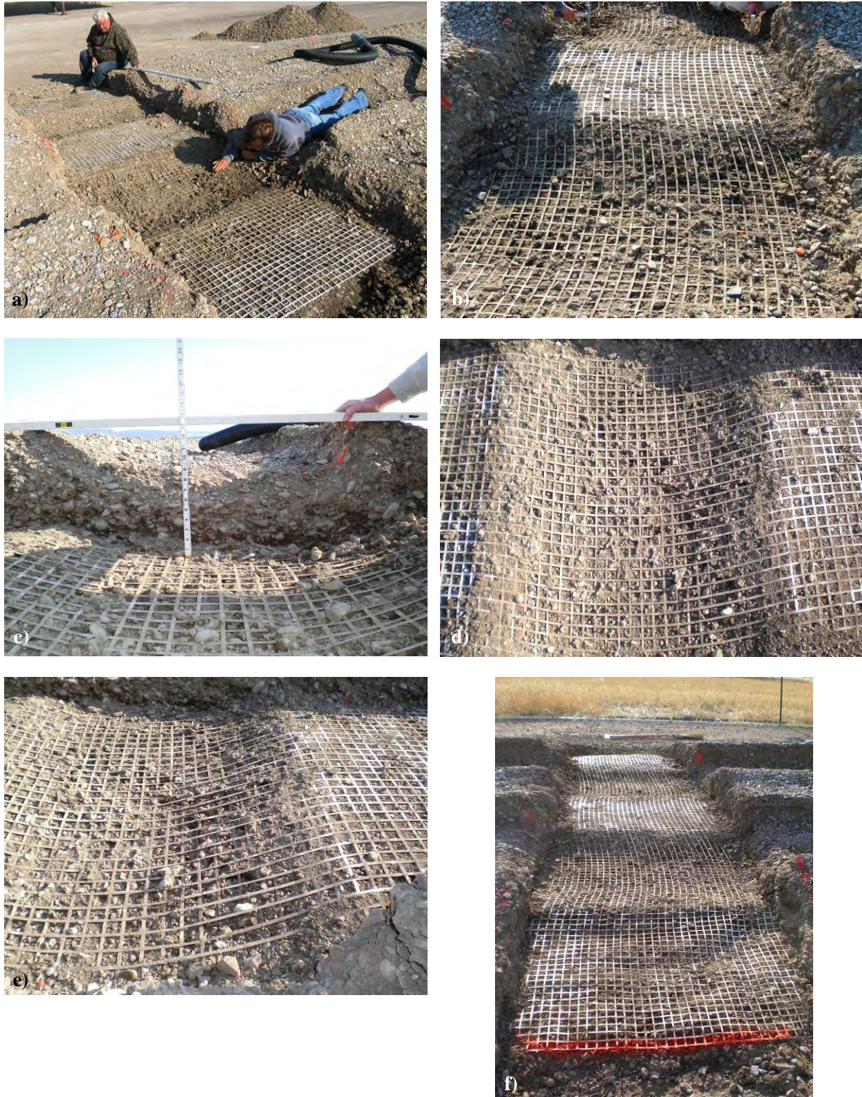
Figure C-11. Photos of the forensic excavations of the WeG-2 test section: a) looking east, b) rut bowl, c) close-up of rut bowl, d) overhead view of rut, e) close-up of rut, and f) looking west.
