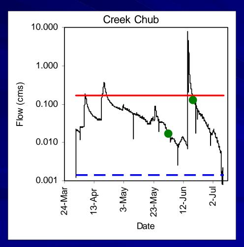
b) FishXing indicated that a passage window exists and fish are observed to not pass the culvert at flows outside that window
