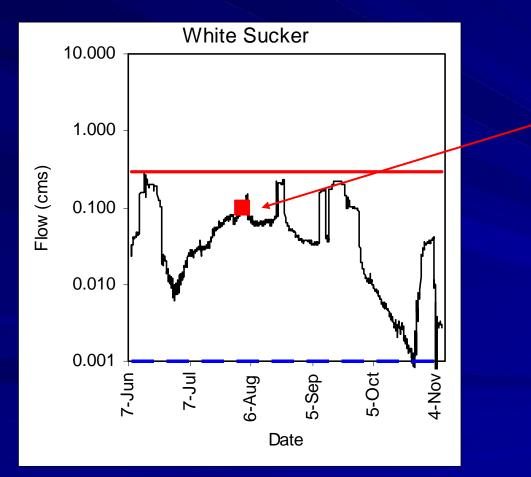
Passage window predicted by FishXing, but fish observed to not pass culvert, an example of case e)
