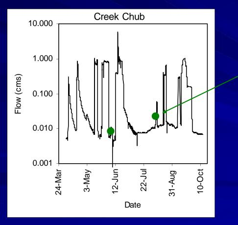
No passage window predicted by FishXing, and fish were observed to pass culvert.
