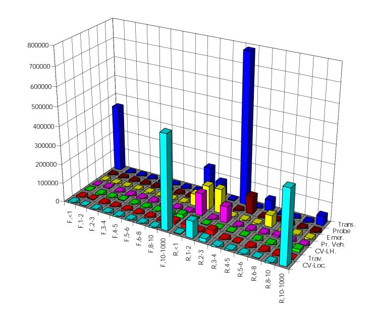
Note: Y-Axis = Number of messages in peak period; X-Axis = Message (in hundreds of bits); F=Forward Direction; R=Reverse Direction
