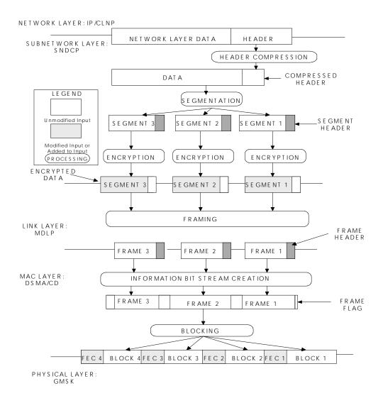
Figure 7.5-5 CDPD Protocol Stack (CDPD System Specification, Release 1.0)
