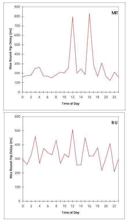
Figure 7.5-39 Example of the Range of Round-Trip Delays (Boston, March 5-7, 1996)
