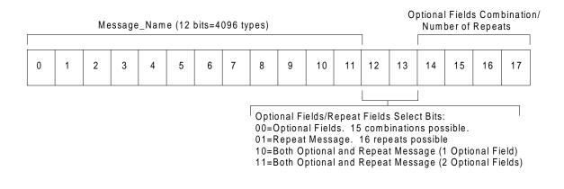
Figure 5.2-2 Details of the Message\_ID Field which Allows Standard, Optional, and Repeated Fields to be Appended to the Message
