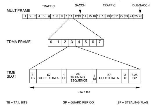
Figure 7.5-9 GSM Frame and Slot Structure
