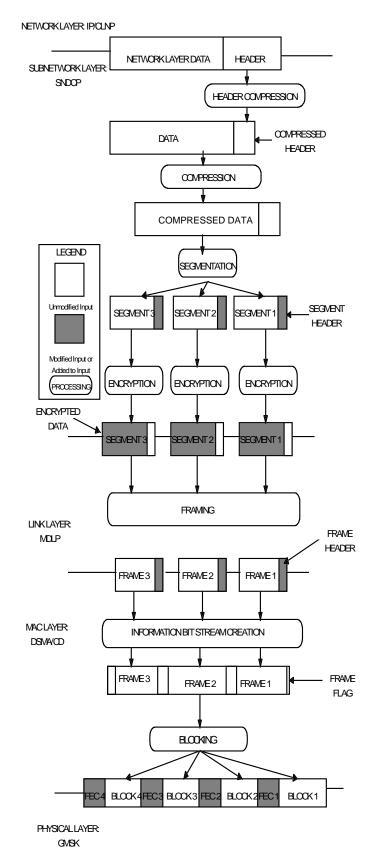
Figure 7.5-6 CDPD Protocol Stack (CDPD System Specification, Release 1.1)
