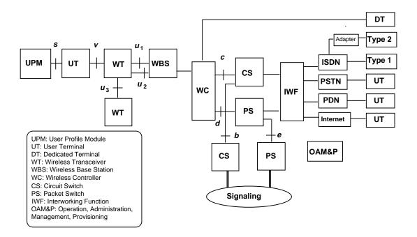
Figure 3.1.-3 Network Reference Model for the Communications Layer
