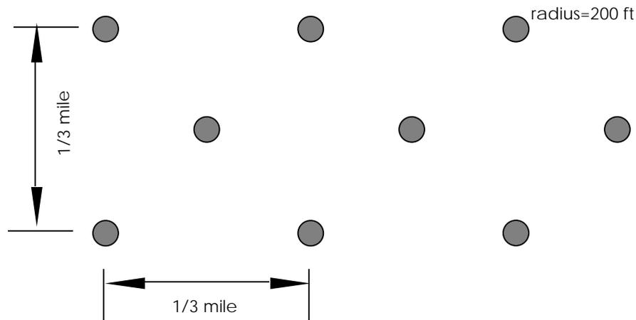
**Figure 7.5-34 Full Deployment of a Beacon System**
