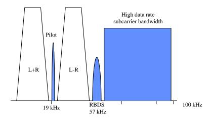
Figure 7.5-26 FM Baseband Spectrum (Not to scale)
