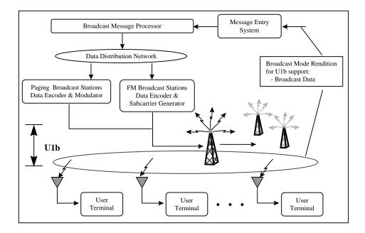
Figure 3.2-7 Rendition 1 for Wide-Area One-Way Wireless (u1b) Links
