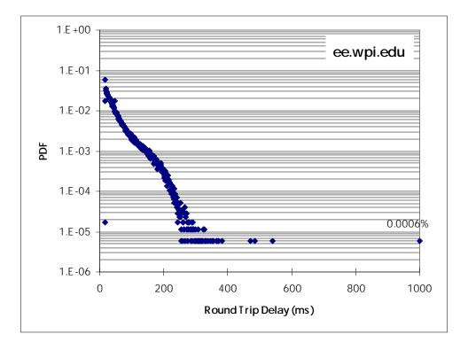
Figure 7.5-37 PDF's of the Round-Trip Delay (Cont.)
