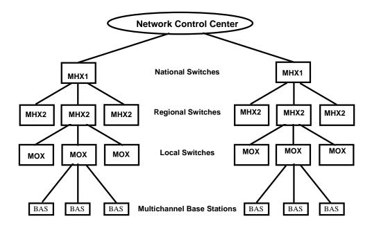
Figure 7.5-12 MOBITEX Network Architecture
