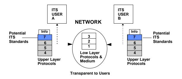
Figure 3.1-1 Generic Hierarchical Communication Model
