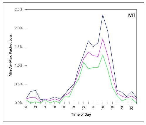
Figure 7.5-40 Minimum-Average-Maximum Packet Loss (Boston, March 5-7, 1996)
