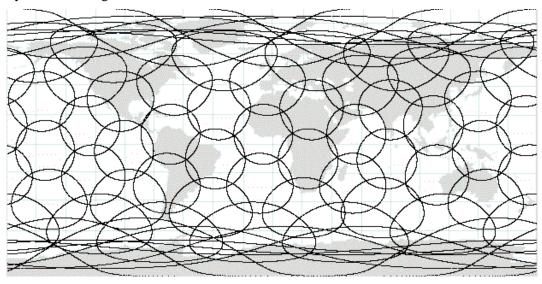
Figure 7.5-15 Iridium System Footprint at a Given Point in Time
