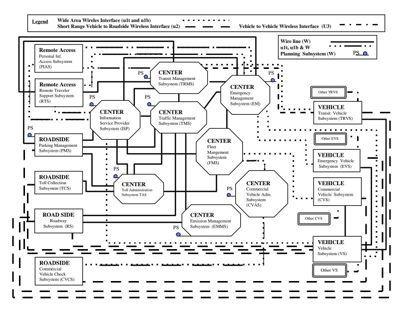
Figure 3.2-3 Level 0 Architecture Interconnect Diagram for the National ITS Architecture
