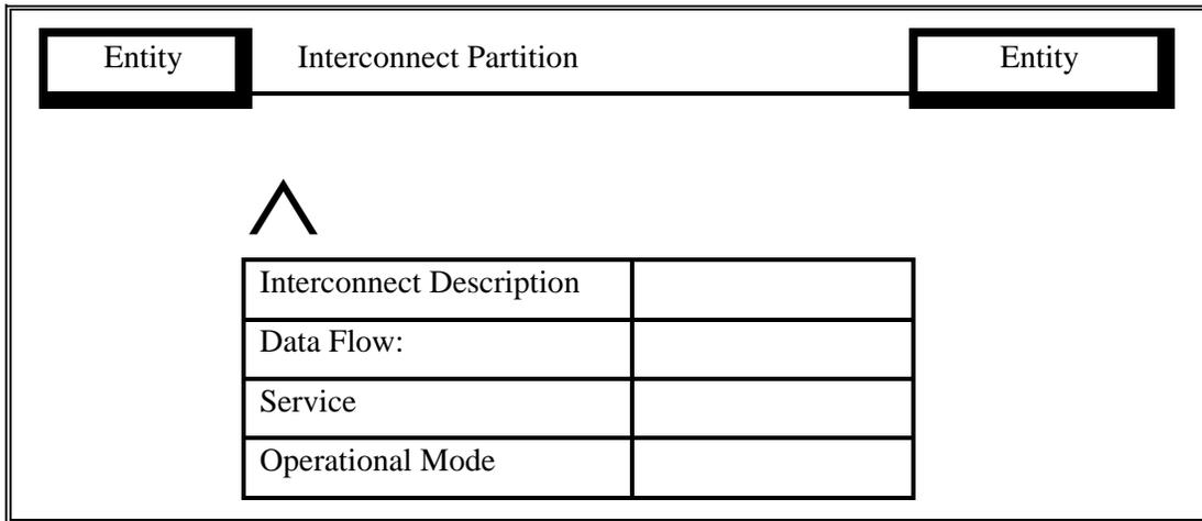
**Figure 3.2-1. Template for the Architecture Interconnect Diagram (AID)**
