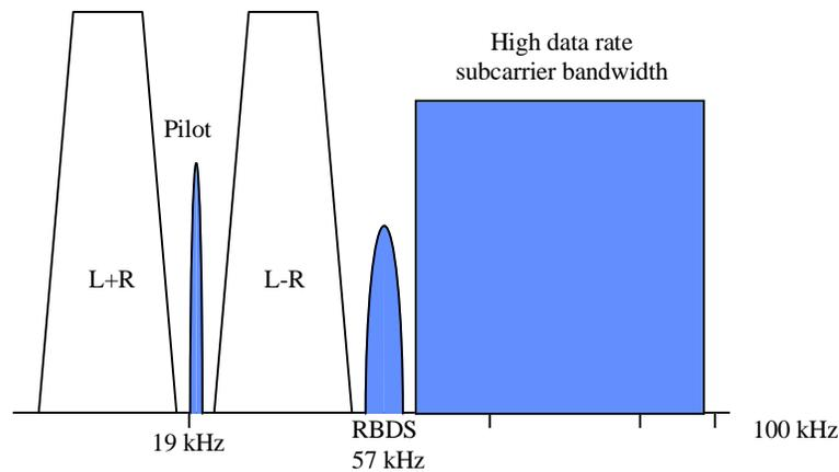
**Figure 7.5-26 FM Baseband Spectrum (Not to scale)**
