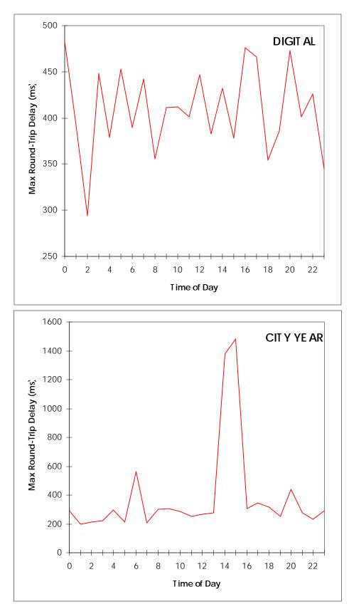
Figure 7.5-39 Example of the Range of Round-Trip Delays (Boston, March 5-7, 1996) (Cont'd)
