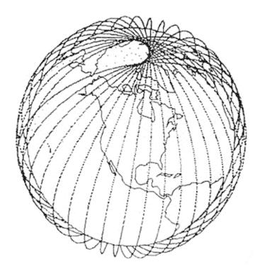
Figure 7.5-16 Path Described by a Teledesic Satellite
