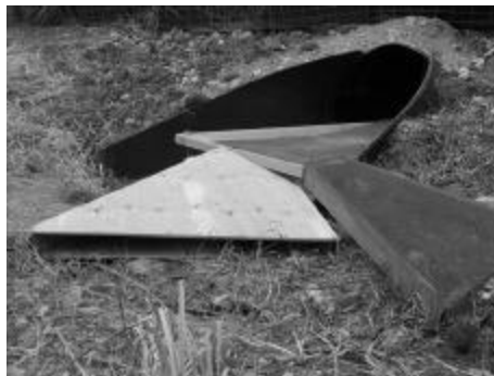
Figure 17. Appearance of entrance funnel entering from side (plywood model in middle of photo). [Compare this prototype to the final design illustrated in Fig. 18b where the funnel is incorporated in to the entrance ramp]
