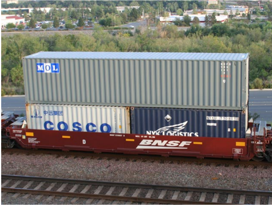
Figure 5: Containers Stacked on a Rail Car (ICWP 2008).
