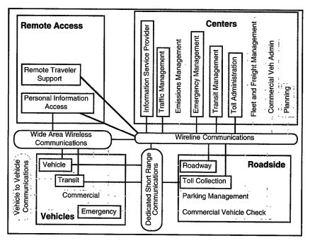
This diagram (Courtesy of the Rockwell/Loral Architecture team), is referred to by the architects as the "sausage diagram" (due to the shape of the communication linkages. It depicts the 19 subsystems for the full ITS and shows the basic communication channels between these subsystems. The highlighted subsystems (i.e., in boxes with bold outlines, such as **Remote Traveler** Support) represent the subset which support the ITI.
