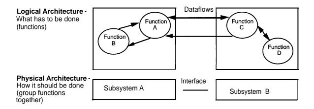
The Logical Architecture documentation defines the DFDs and P-specs. The Physical Architecture Documentation defines the subsystems, assigns P-spec functions to them, and documents the dataflow interfaces between the subsystems. In this document, the architecture subsystems and dataflows needed to implement IT1 are found in Chapter 4.
