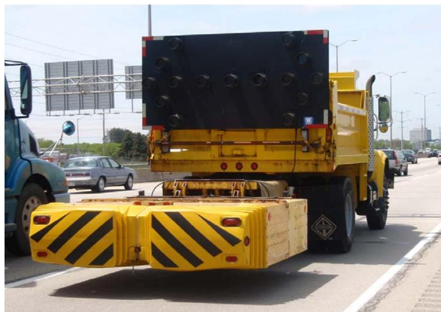
Figure 3. A typical truck-mounted attenuator and arrowboard used for moving lane closures.
