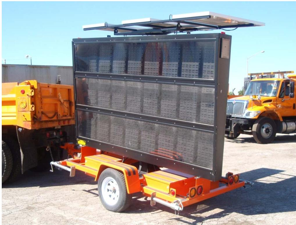
Figure 6. A trailer-mounted PCMS in transport mode.
