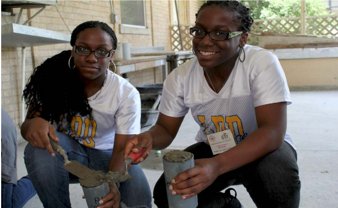
Figure 17. Scholars Preparing Concrete Specimens for Testing
