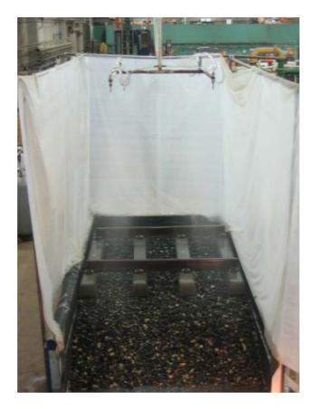
Figure 2. The overall model during a rainfall simulation event.
