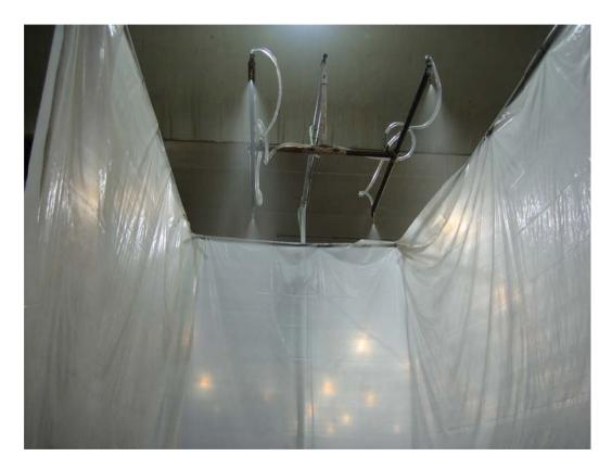
Figure 4. The rainfall simulator with 4 spray nozzles.
