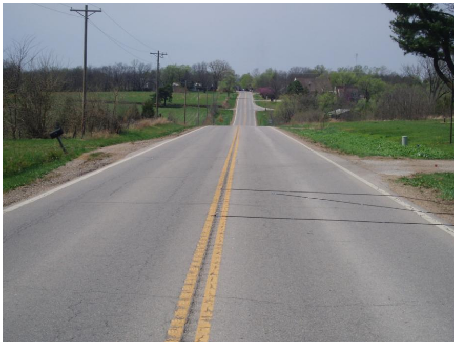
FIGURE 6.4 Set up of Road Tubes Sensors for Data Collection in Section with CLRS
