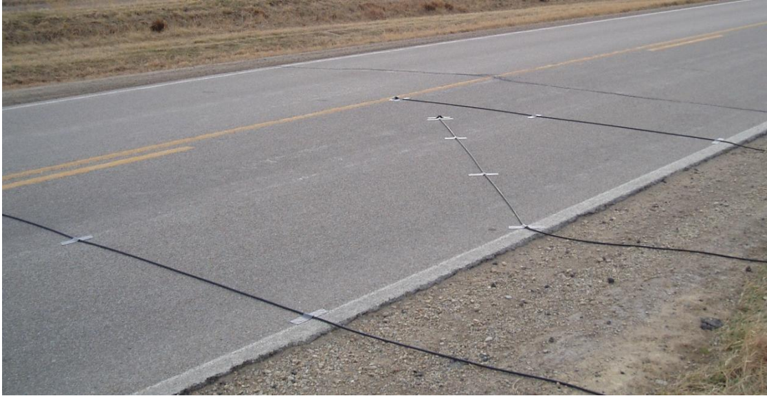
FIGURE 6.5 “Z” Configuration of Sensors for Data Collection
