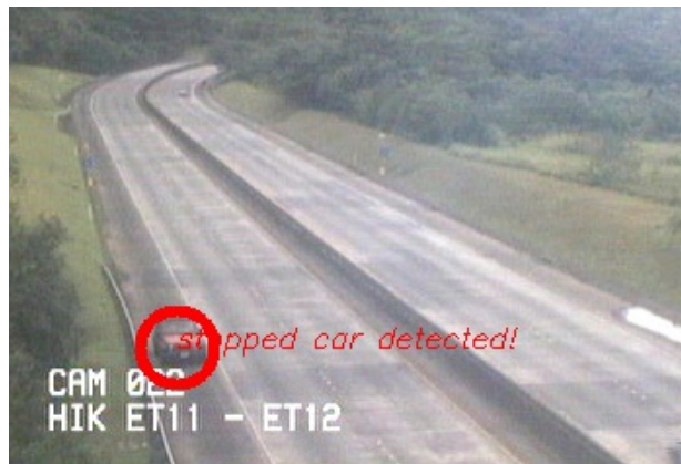
Figure 64 Detection of a Stopped Vehicle
