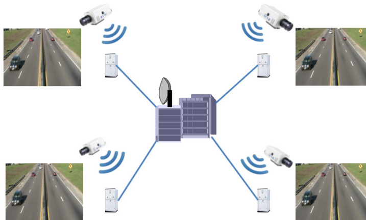
Figure 5 Infrastructure-connected Camera Configuration
