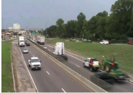
Figure 63 Illustration of Side Occlusion of Two Rightmost Lanes
