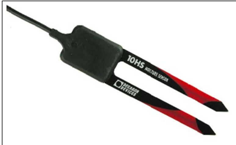
Figure 3-19: Decagon 10HS Soil Moisture sensor (Decagon Devices, Inc., 2012)
