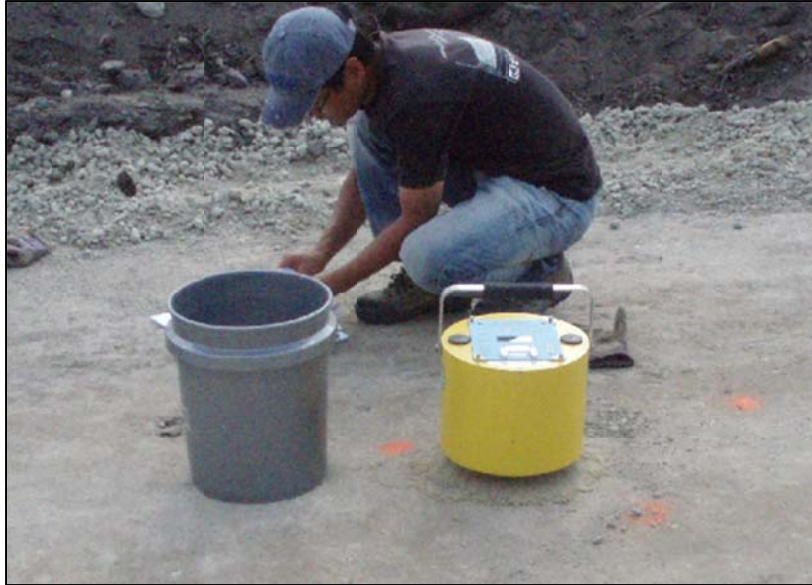
Figure 3-32: SSG test being performed prior to full-scale testing
