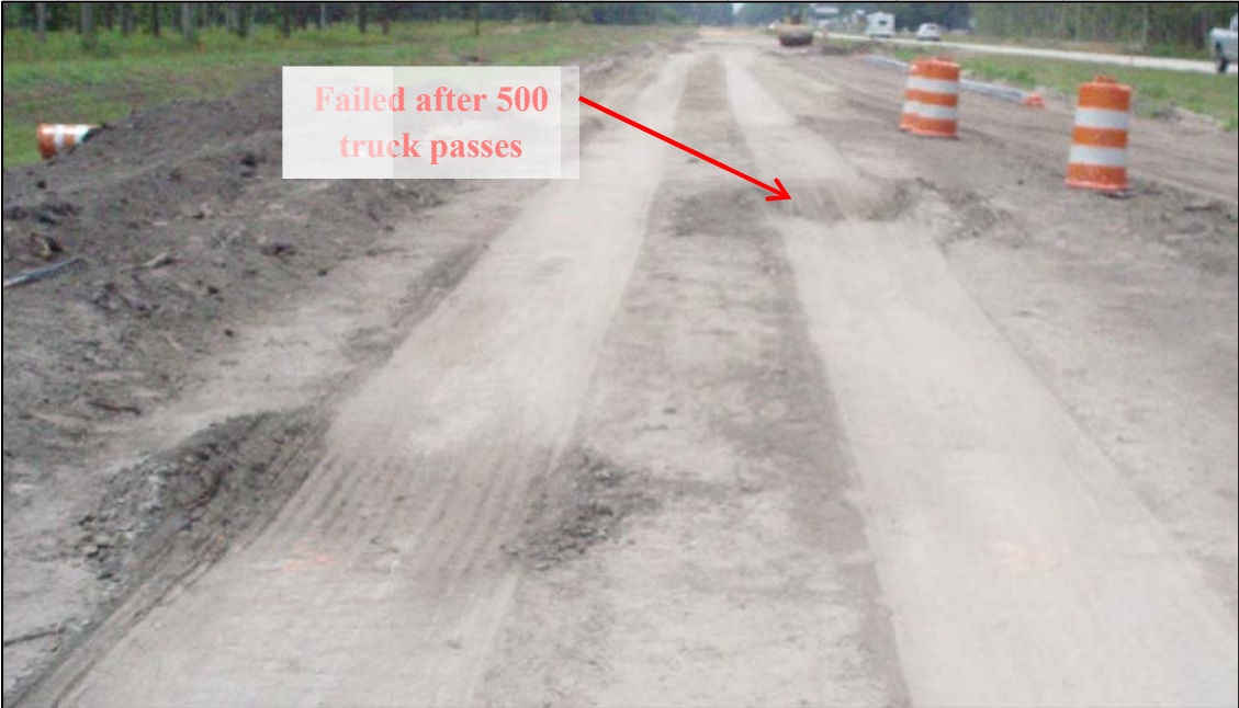
Figure 5-82: Test Section 4 after 1000 truck passes
