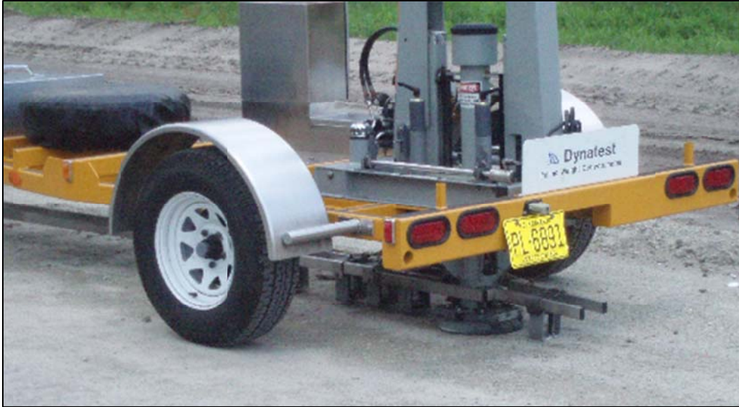
Figure 3-33: FWD testing performed after full-scale testing
