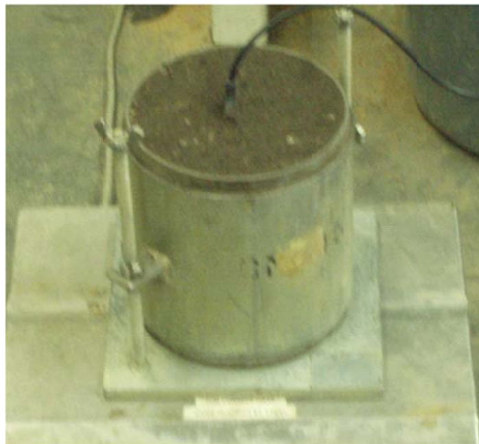
Figure E134: Soil moisture sensor calibration setup
