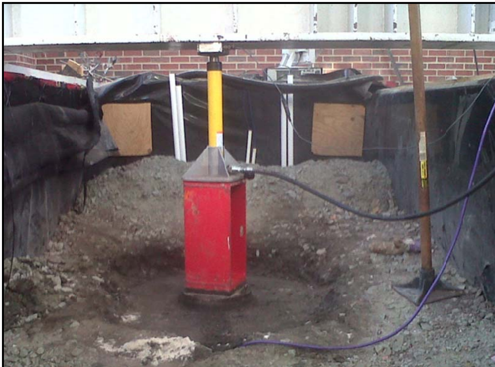
Figure D129: EPC laboratory calibration test setup
