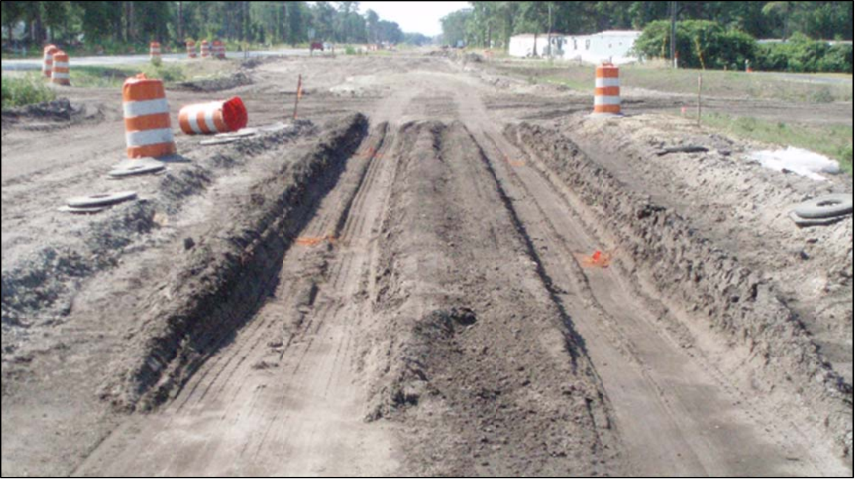
Figure 5-75: Test Section 1 after 200 truck passes
